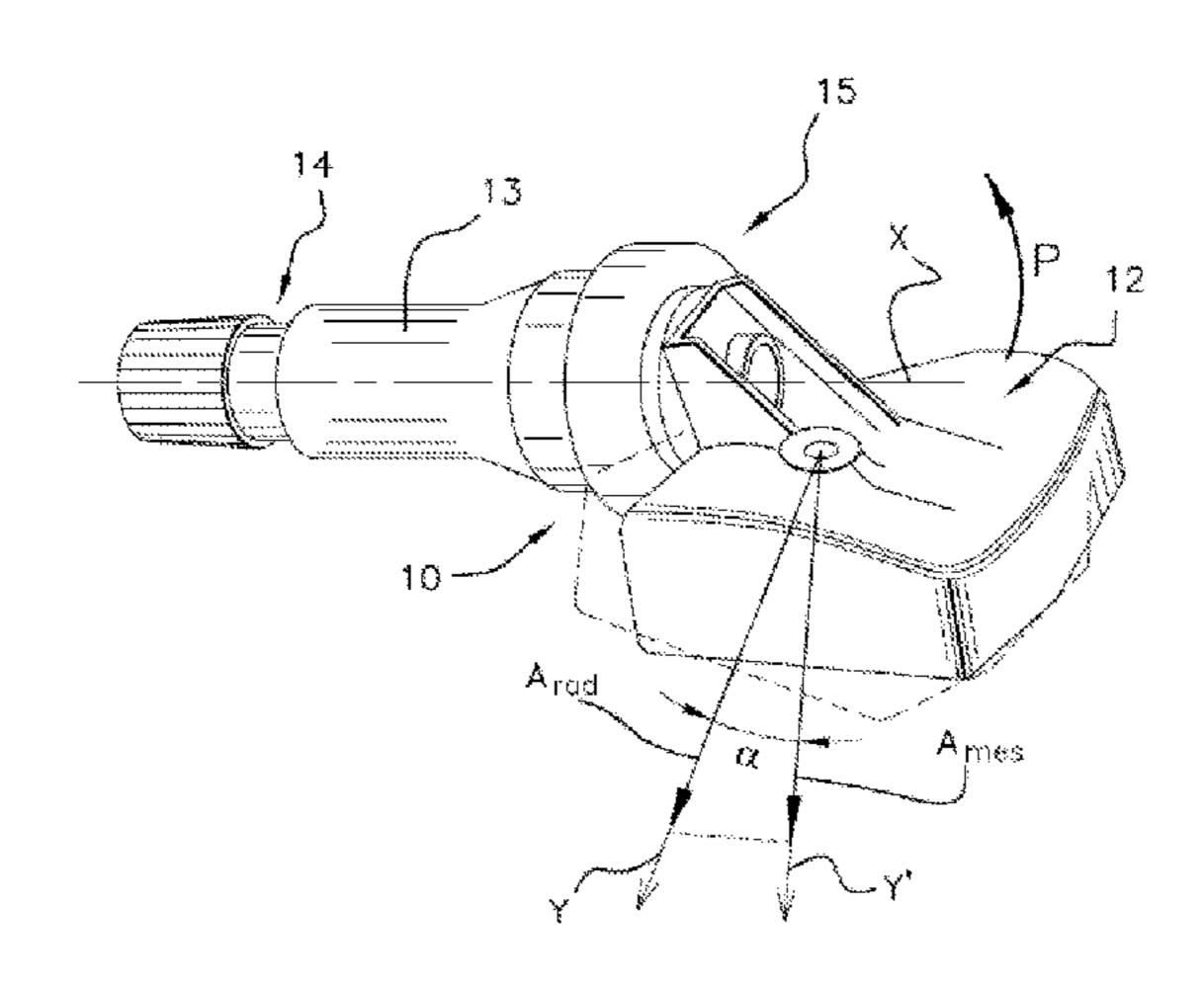
where  $\omega$  is the actual angular speed deduced from the observation of the curve,  $\overline{A_{mes}}$  is a mean value of the corrected radial acceleration, and R is a standardized radius of the wheel.
