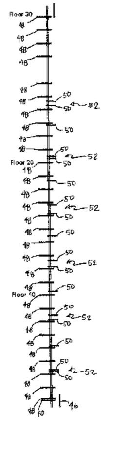
plurality of dummy position indicators (50). The plurality of landing position indicators (48) and the plurality of dummy position indicators (50) are positioned to form a sequence of unique patterns. The position determining system is more cost effective and timesaving than the absolute position reference systems.
