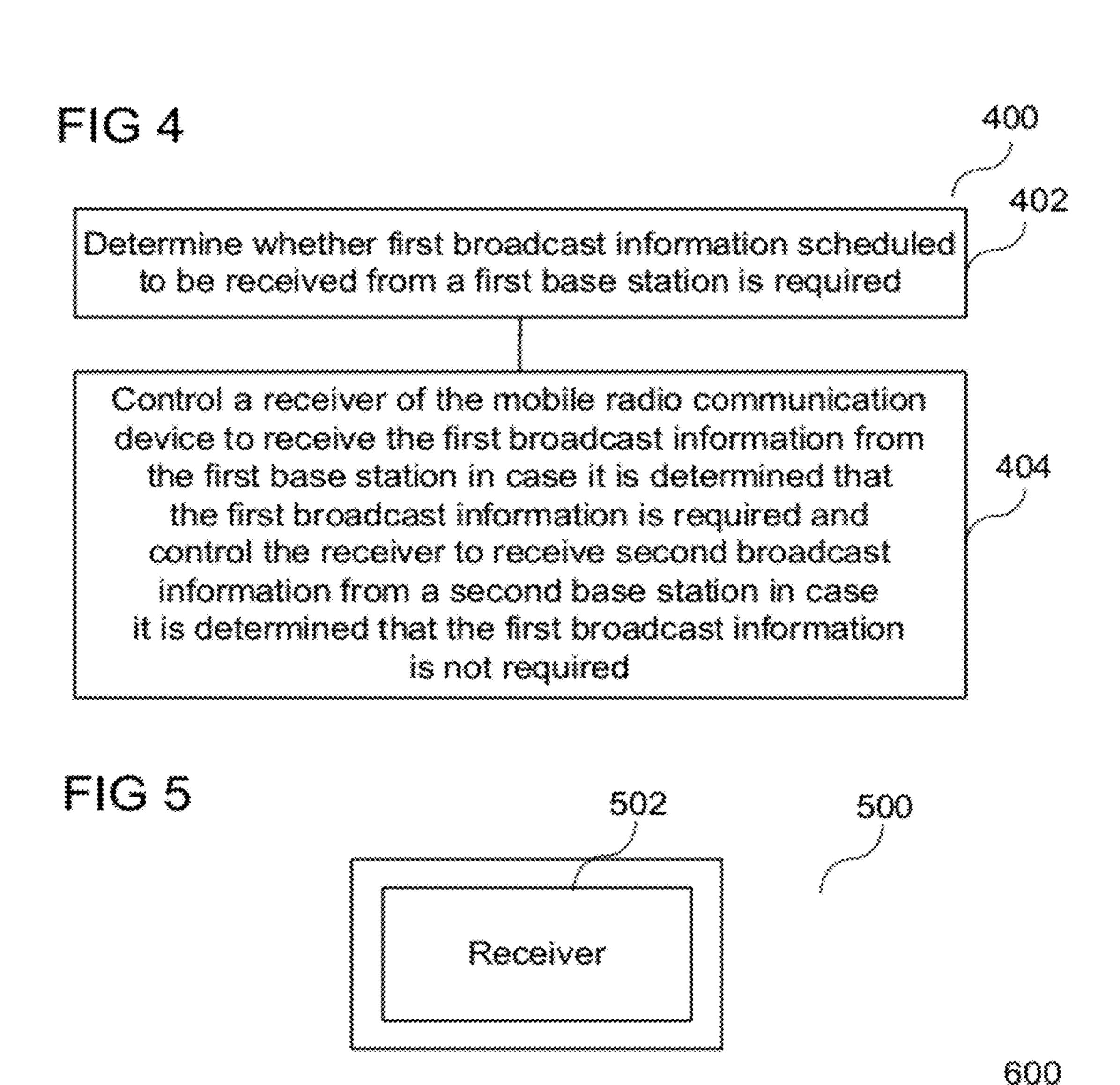
Receive broadcast information from a second base station in case it is determined that broadcast information scheduled to be received from a first base station is not desired by the mobile radio communication device, and receive broadcast information from the first base station otherwise
