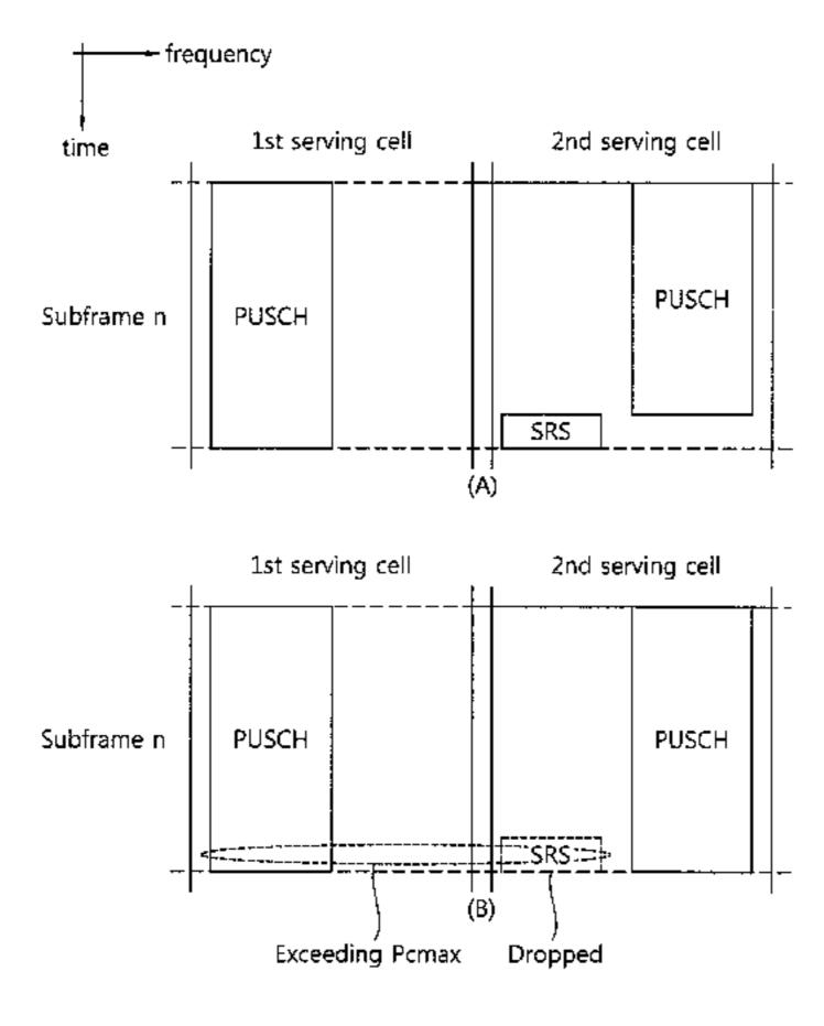
configured to the UE, the UE transmits the PUSCH on the SRS subframe for the first serving cell.
