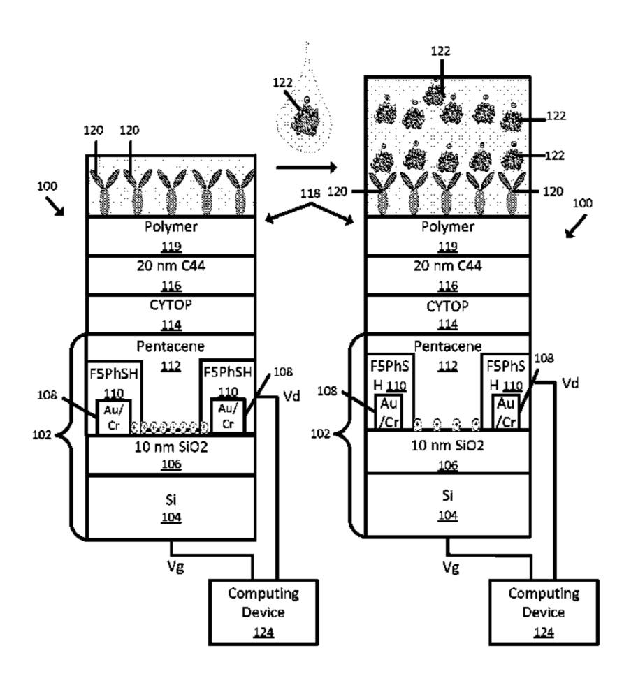
layer. The system also may include a receptor-attachment material configured for binding to an analyte. A receptor may bind to the analyte, and the receptor may be attached to the receptor-attachment material. The binding of the analyte to the receptor can cause the change of the electrical property at the surface. In response to the change for example, a current may change for indicating the binding of the analyte to the receptor.
