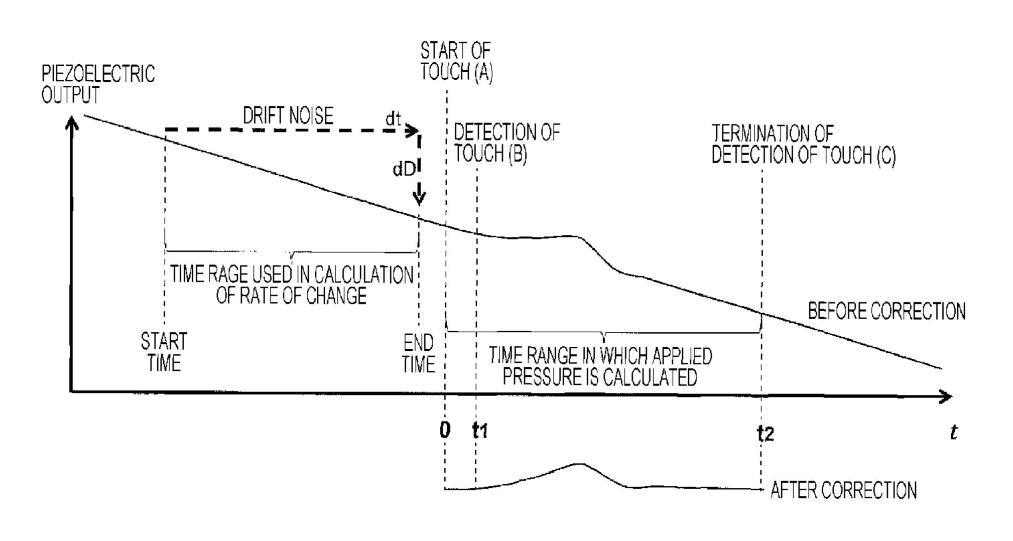
with the pressure sensor. An applied pressure calculator calculates applied pressure by correcting the piezoelectric output acquired after an end time of the time range used in the calculation of the rate of change using the rate of change. The apparatus enables precise measurement of applied pressure in a pressure sensor.
