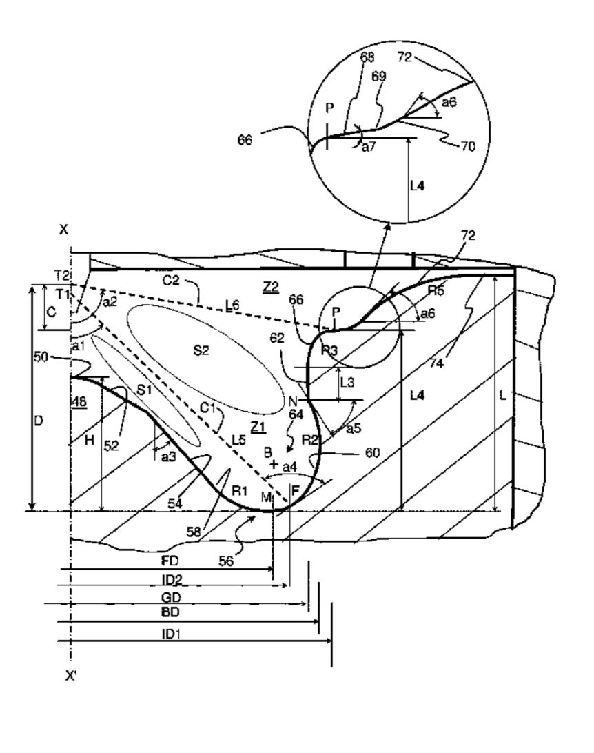
jecting fuel in at least two fuel jet sheets with sheet injection angles (A1, A2), a lower sheet (36) of jet axis C1 and an upper sheet (38) of jet axis C2, at least two mixing zones (Z1, Z2) of the combustion chamber. According to the invention, one of the zones comprises a toroidal volume (64) of center B into which fuel jets (40) of the lower jet are injected in such a way that axis C1 of the lower jet is contained between center B and projection (48).
