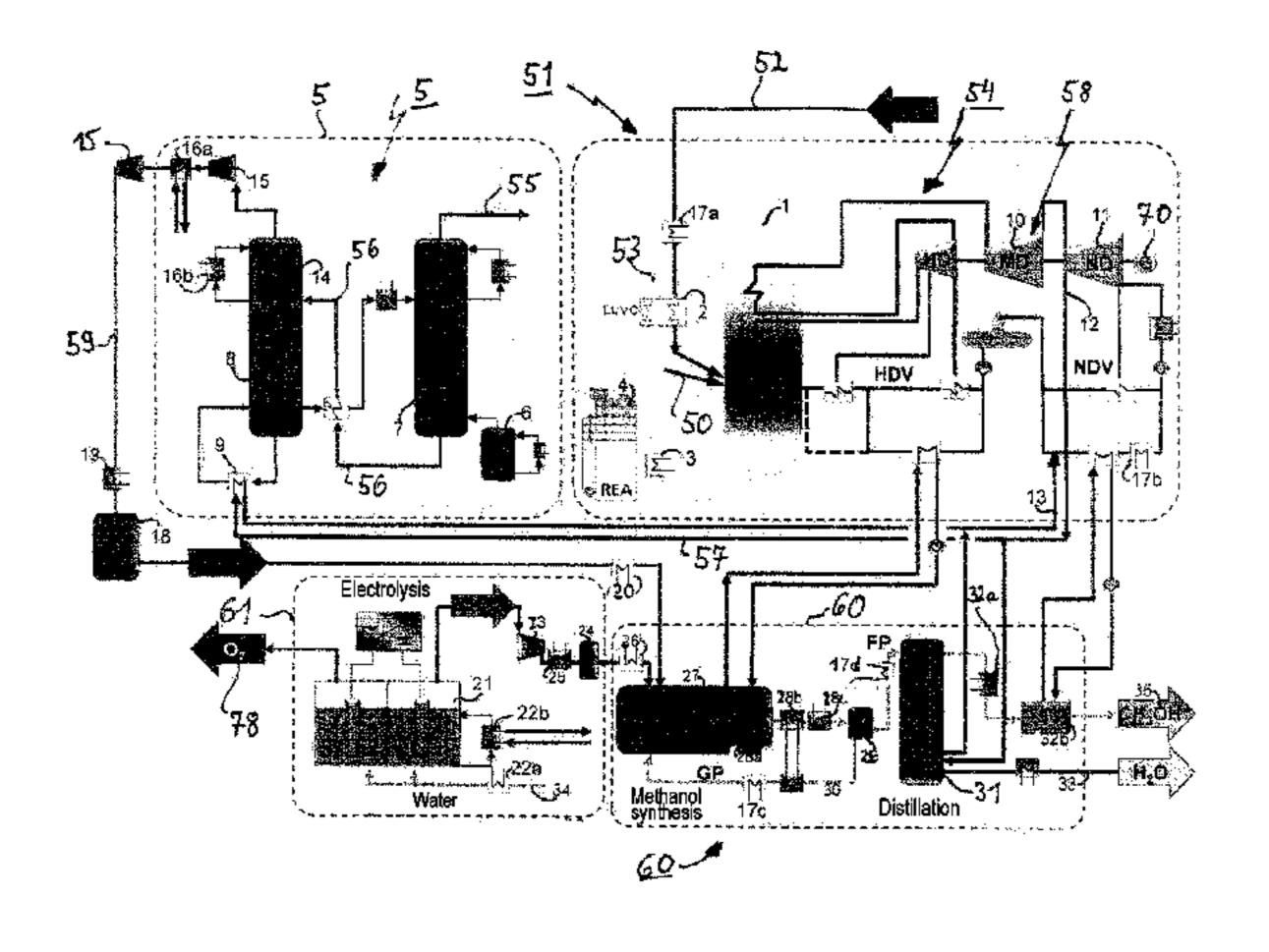
plant that is fired with hydrocarbon-containing fuel, which operating method permits in particular a rapid adaptation of the power plant output to the power demands from the grid.
