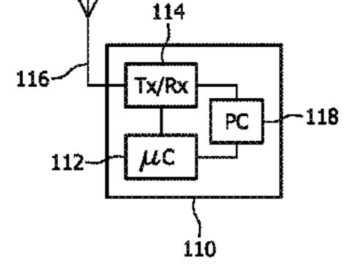
secondary station deduces from the part of the search space used for transmitting the control message an indication of the resource set from the plurality of resource sets within which the allocated resource is located.
