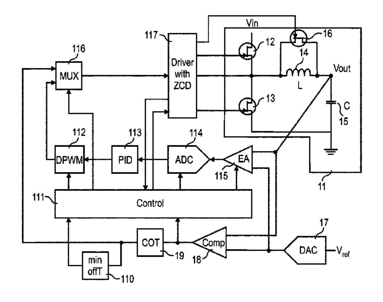
control path when the multi-mode controller is run in a light load mode.
