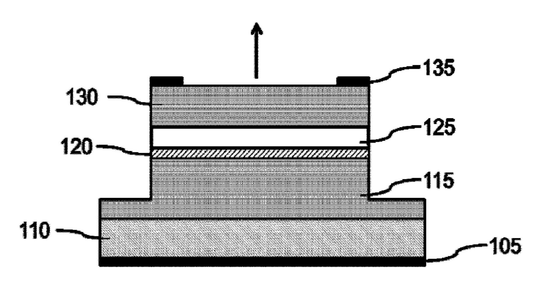
provide a VCSEL which can be easily and reliably processed by integrating the distributed heterojunction bipolar phototransistor (125, 425, 625, 725).
