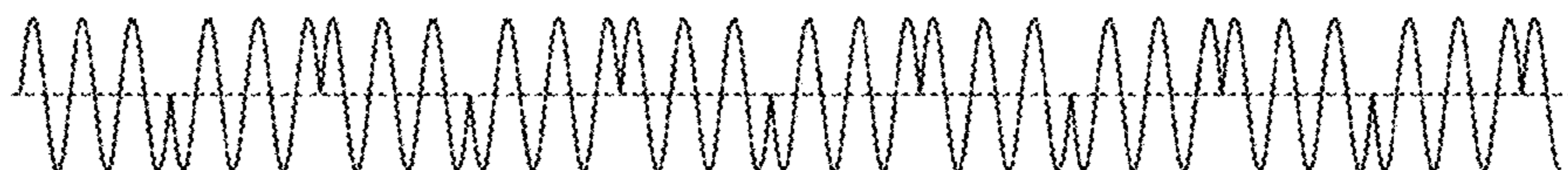
AC COMPONENT OUTPUT BY AC POWER SUPPLY UNIT
