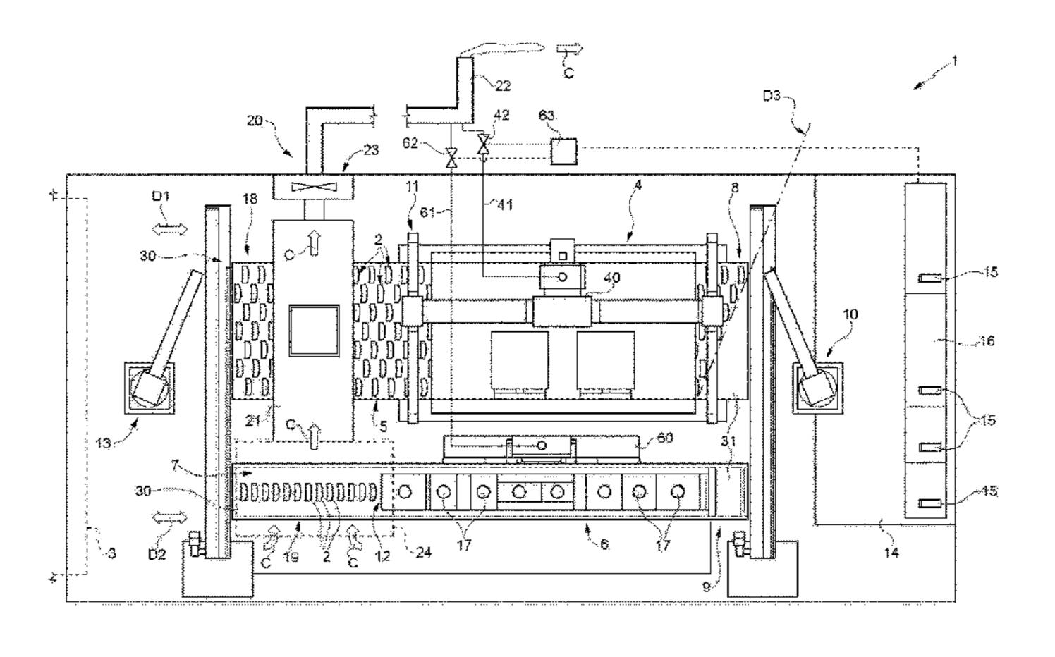
veyor belt to the second one or vice versa to a first end of the furnaces and place them on the first conveyor belt or second one to a second end of the furnaces being opposite to the first one, so as to change at will the sequence in which the infrared and convective heating steps are performed.
