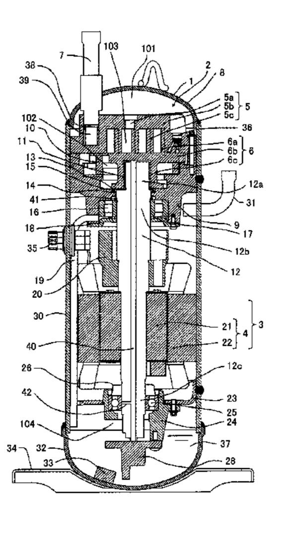
portion and the bearing part, in contact with the flange portion on the upper side and in contact with the bearing part on the lower side. Assuming that the outer diameter of the flange portion 12d is  $\varphi Dt$  and the outer diameter of the thrust stopper is  $\varphi Ds$ ,  $\varphi Dt < \varphi Ds$  holds.
