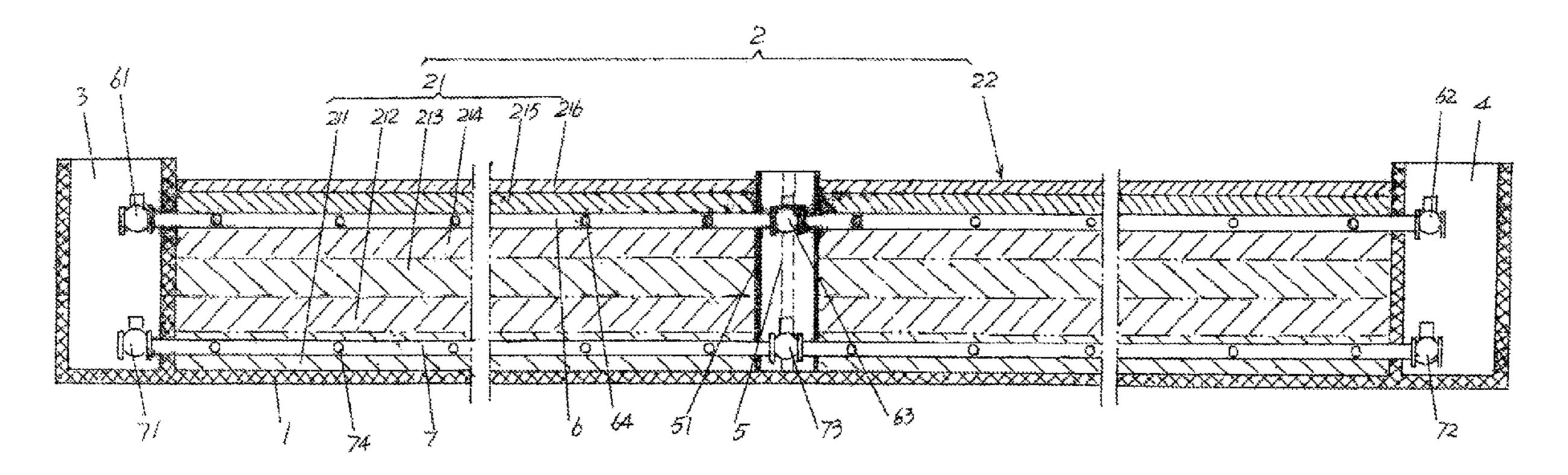
water conduit inlet valve at one end. It ensures the service life of the vertical flow sewage treatment artificial wetland and avoids pipe blockage; has the lasting purification treatment capacity; has a simple structure and can achieve the low cost of construction and convenient operation management; and has a long-term stable use effect.
