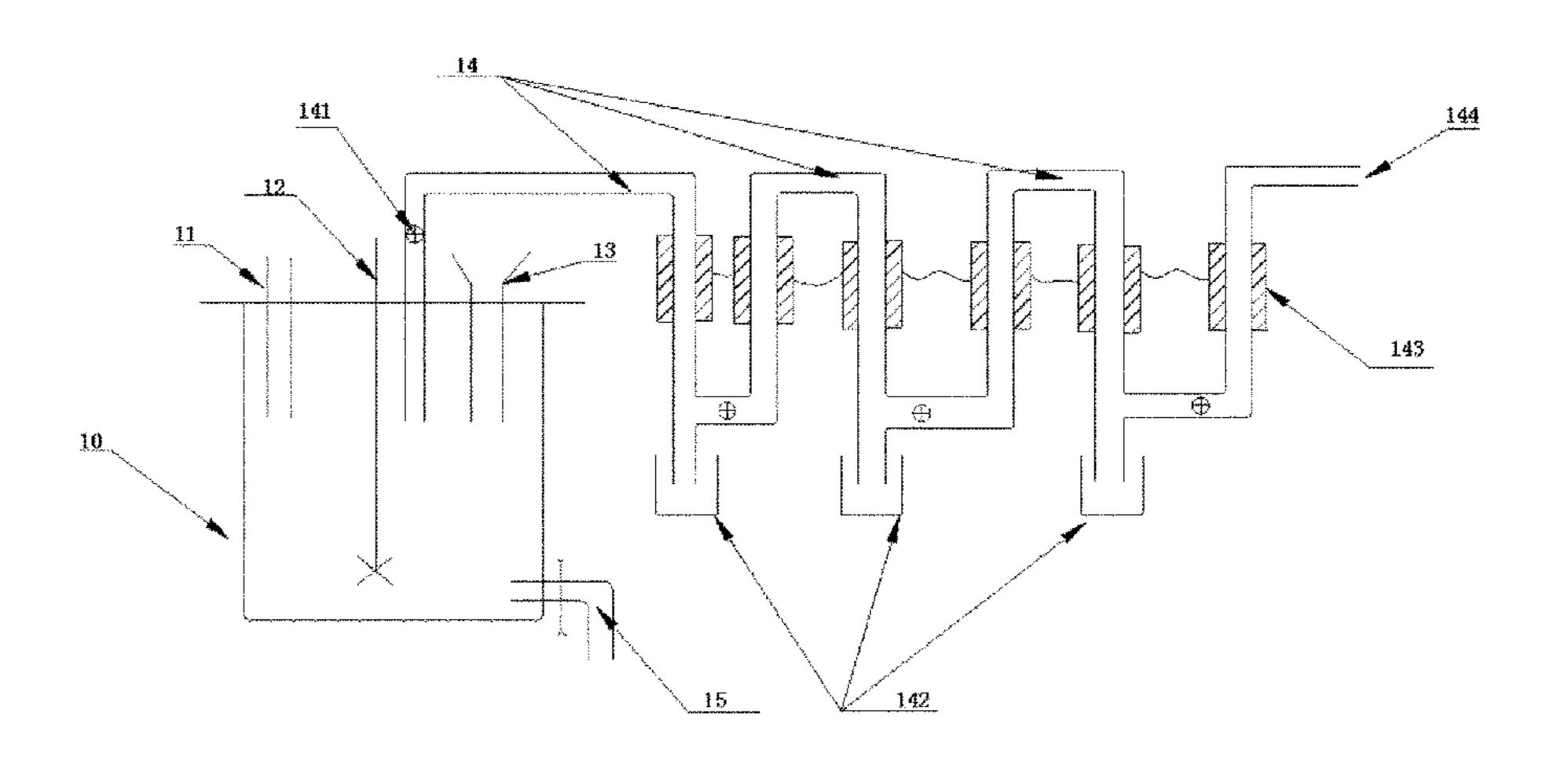
oxidize Fe<sup>2+</sup> into Fe<sup>3+</sup> and adding K<sub>2</sub>CO<sub>3</sub> solution to clean element Fe out by a form of Fe(OH)<sub>3</sub> flocculent precipitate, and the hydrofluoric acid (HF) can be recycled which can realize the HF zero polluting discharge.
