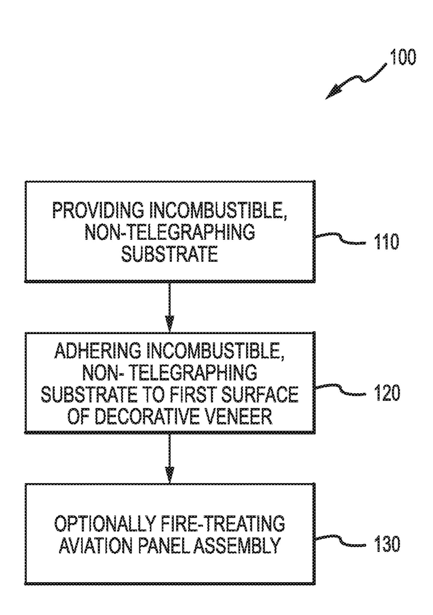
INCOMBUSTIBLE, NON-TELEGRAPHING SUBSTRATES FOR AVIATION PANEL ASSEMBLIES AND METHODS FOR INSTALLING THE INCOMBUSTIBLE, NON-TELEGRAPHING SUBSTRATE INTO AN AVIATION PANEL ASSEMBLY
