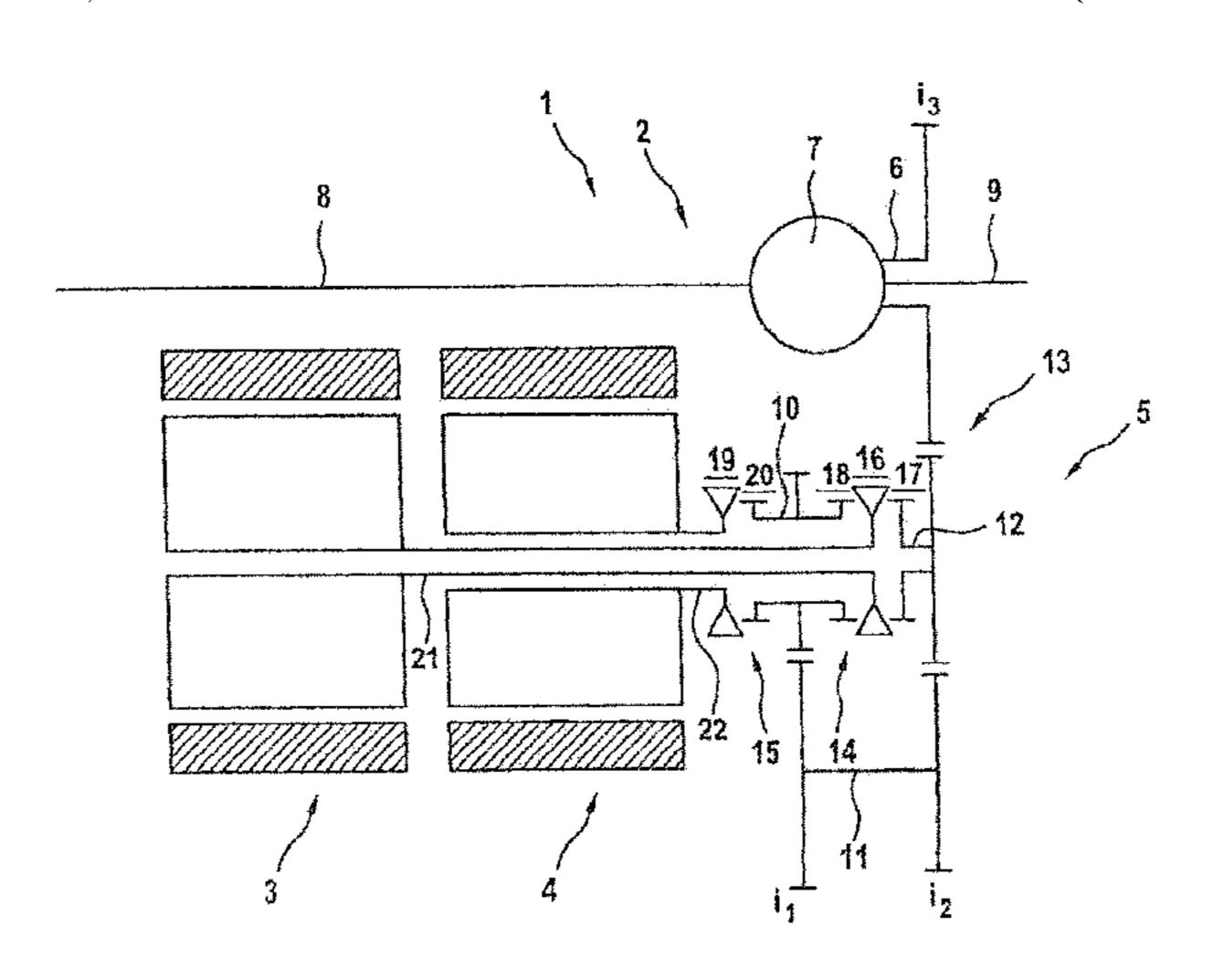
acceleration operating mode and the second acceleration operating mode the operative connection between the first electric motor and the intermediate shaft is interrupted for a defined switching time period. During the switching time period the second electric motor is operated with an overload torque.
