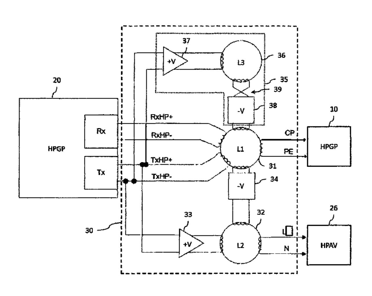
one first coupling transformer, which couples a data transmission device of a charging station to the data transmission devices of the vehicle and of the communications network via respective coils. The signal-matching device is configured to match the first signal level to the second signal level and vice versa.
