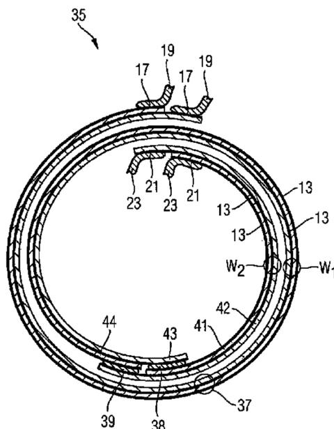
of the coil winding than the contact side of second strip conductor.
