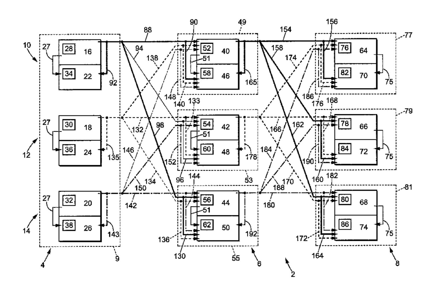
a single unidirectional communication link connecting the control computer of the third piloting control stage to the control computer of the third control-surface position calculation stage.
