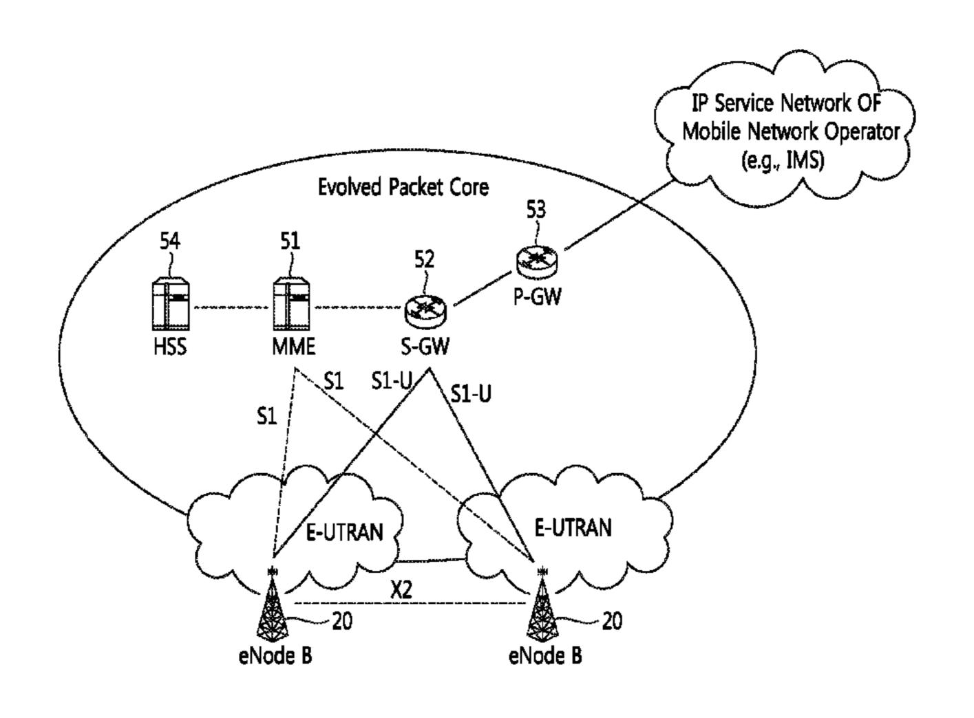
or wireless LAN-based RAT, and a mobility management entity (MME). The method can comprises the steps of: transmitting, by the radio access device, a request message to the MME; and receiving a response message from the MME.
