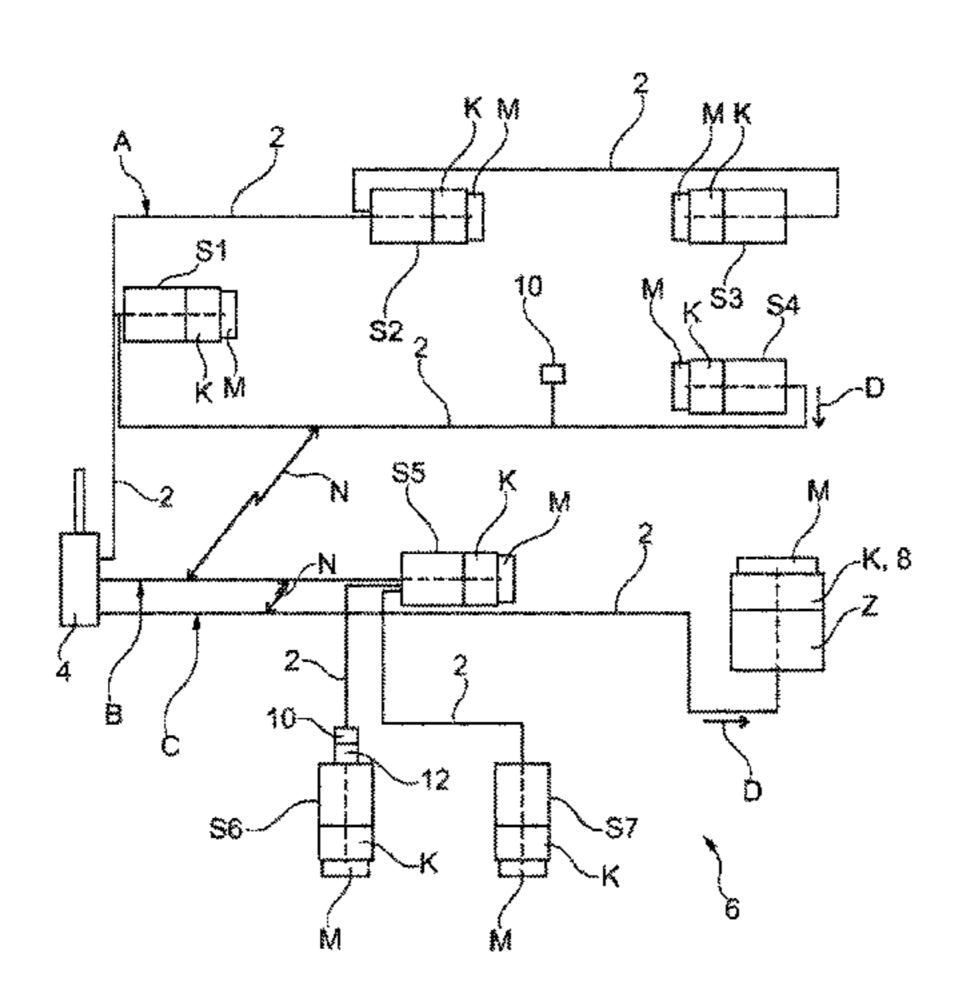
data via the supply lines in combination with the setting up of a partially interlinked data network, signal transmission is made possible even if there is no direct connection between the respective sensor and a target unit.
