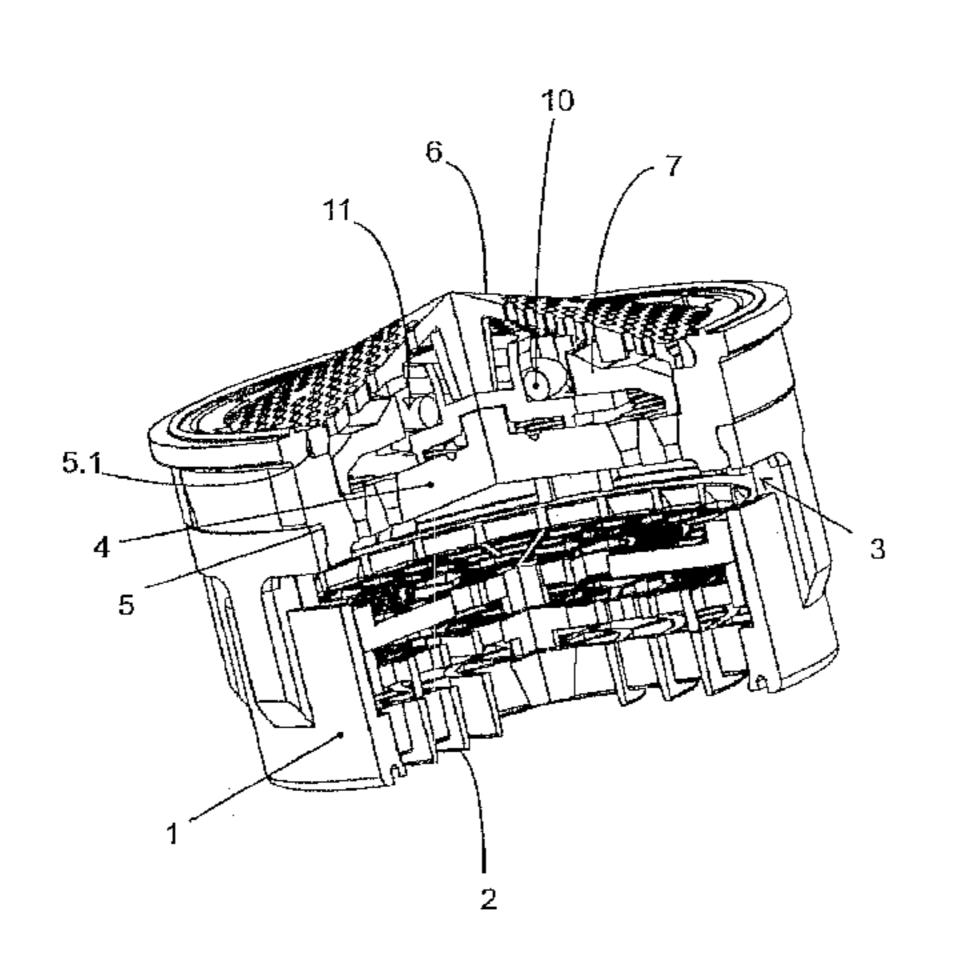
binable so as to realize adaptability to different user and user requirements. A locking means is provided e.g. on the inner circumference of the shell body for this purpose as is a corresponding counter-locking means on the outer circumference of the diffuser plate assembly. The diffuser plate assembly exhibits, at least on its exterior, a flow rate class-specifying optical code and the shell body exhibits a stream type-specifying, namely laminar or aerated, optical code.
