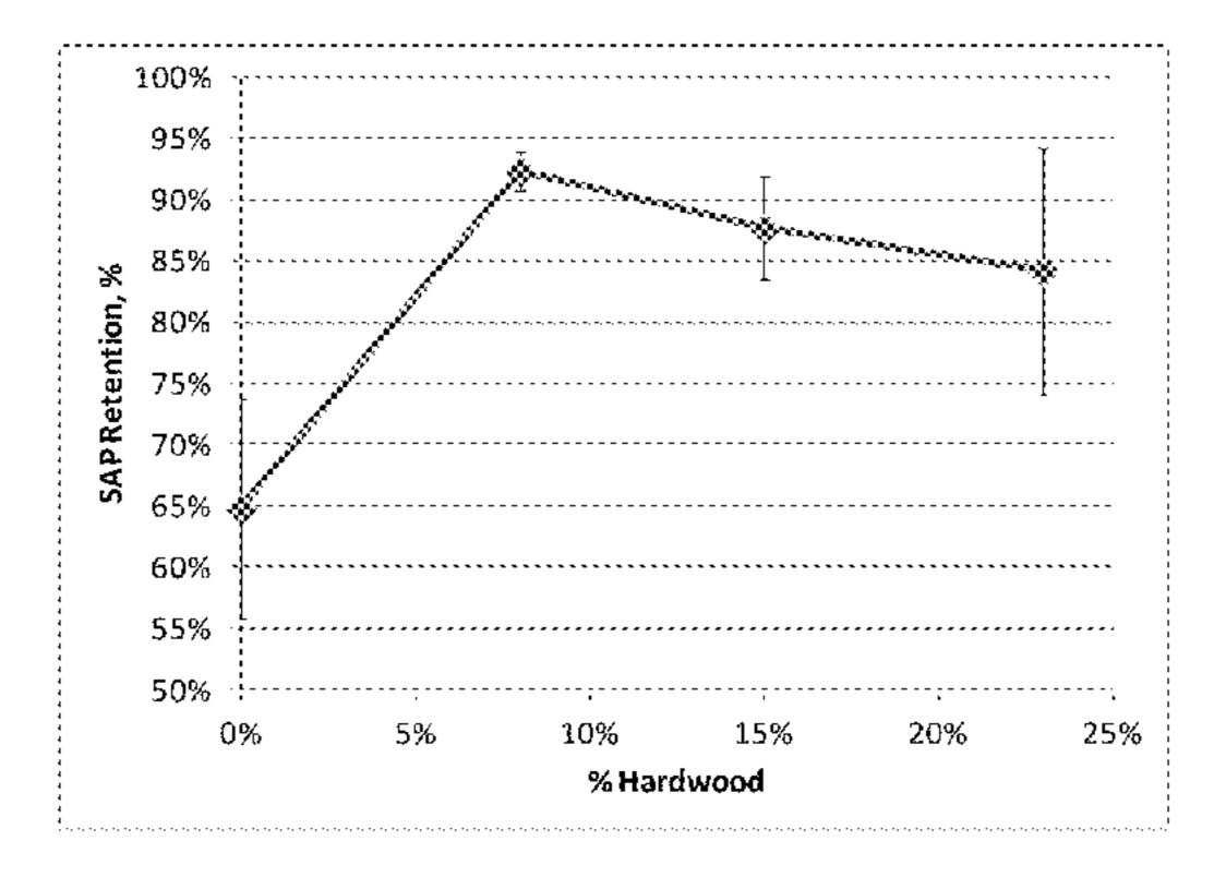
Procedure: Form pad with 50% fluff pulp and 50% SAP. Shake pad on mesh screen. Determine SAP retained by weight difference before and after shaking.
