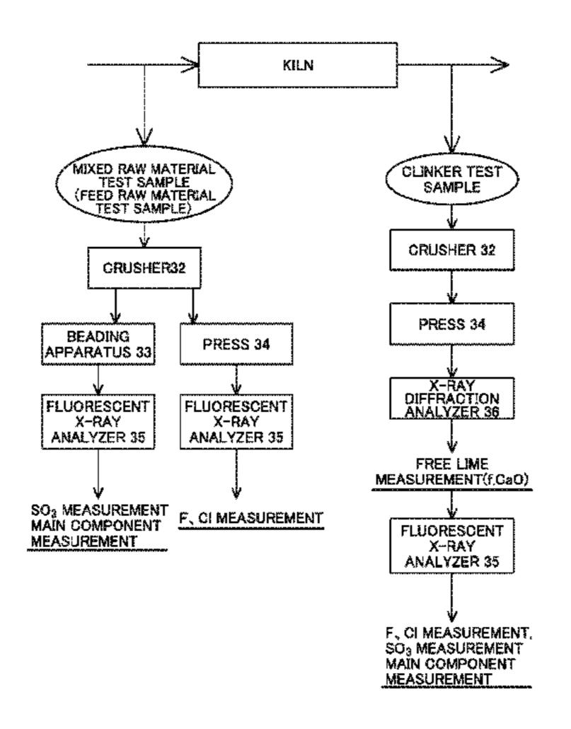
material; an introducing section configured to introduce the sulfur source of the mineralizer to the kiln; a third supplying section configured to supply fuel to the kiln; and a test sample-analyzing system configured to collect each of the mixed raw material before the burning and the clinker after the burning and to measure amounts of the fluorine, main components and free lime depending on the type collected.
