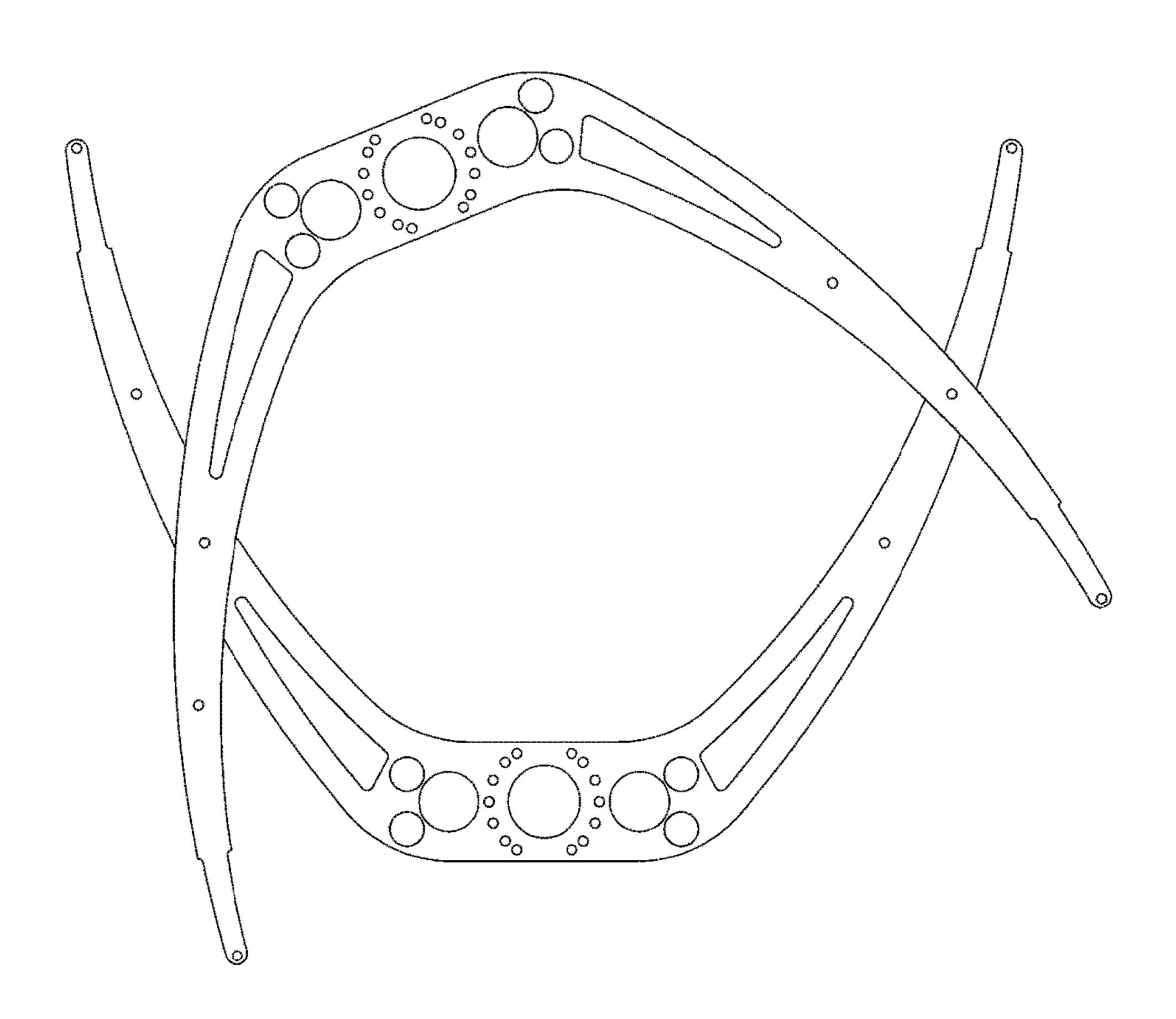
Figure 15. Device as two units attached in an "S" configuration.
