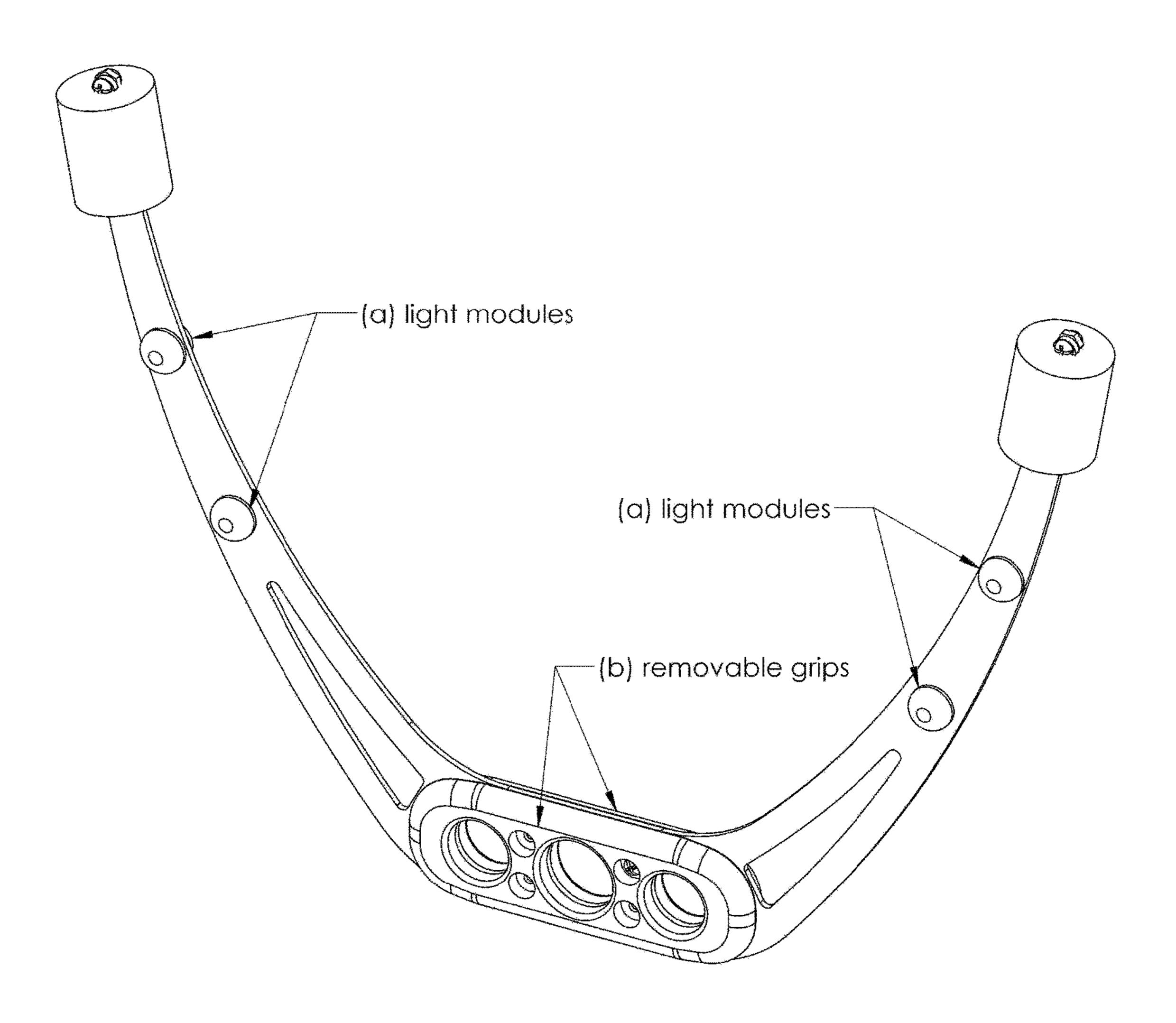
Figure 24. Finger loop bracket.
