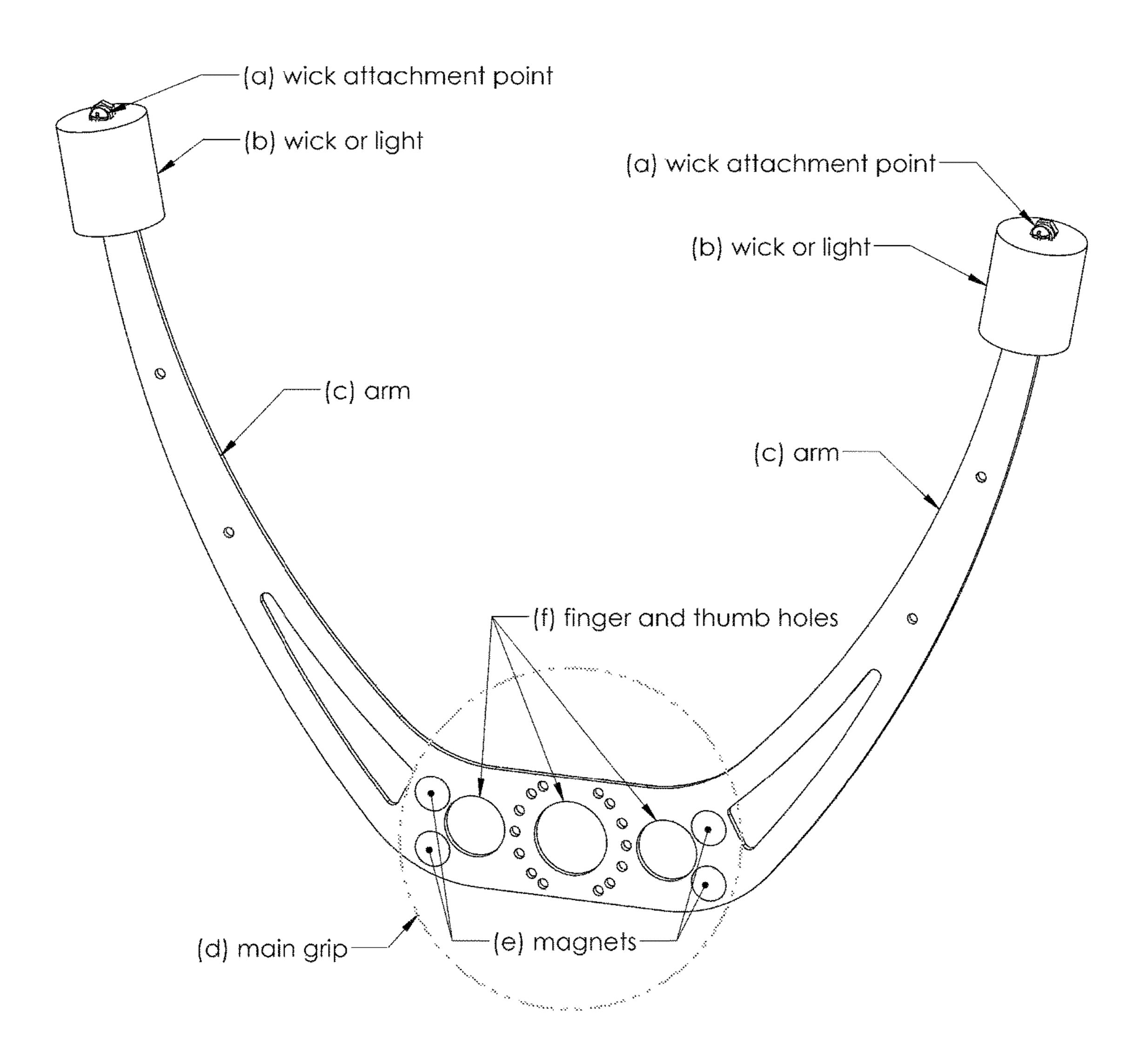
Figure 3. Device as two units attached in a "fan" configuration.
