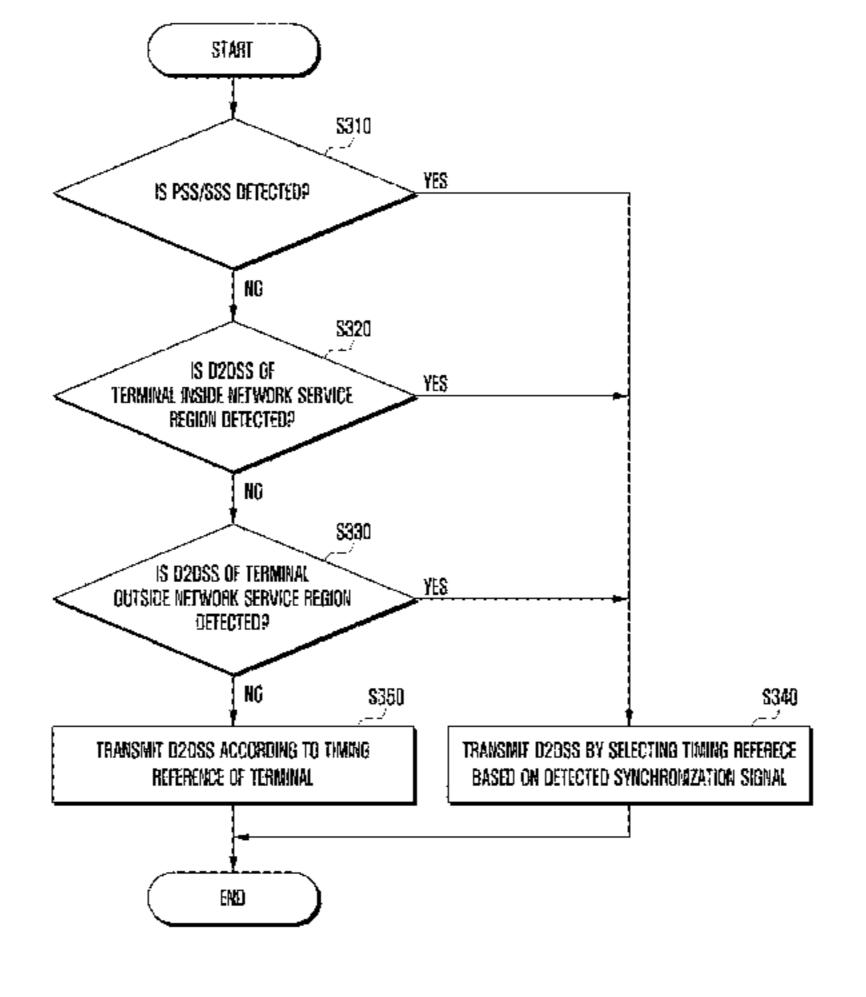
signal is detected, configuring synchronization with the another device based on the timing reference of the detected synchronization signal.
