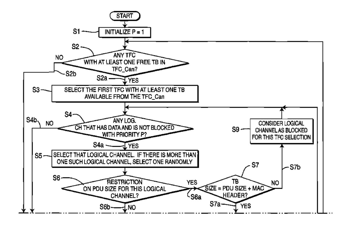
and on the respective first value of each of the logical channels being greater than zero. Also, the controller may multiplex the MAC SDUs of the selected logical channels to produce the MAC PDU. In addition, the controller may provide a transport block for transmission based on the MAC PDU. The controller and a transmitter may then transmit the provided transport block.
