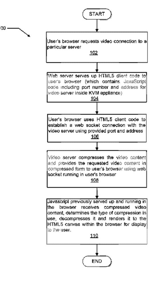
HTML5 client code, the web socket connection and the web socket may be used to receive the compressed video, and the HTML5 client code may be used to decompress the compressed video for display on the personal electronic device.
