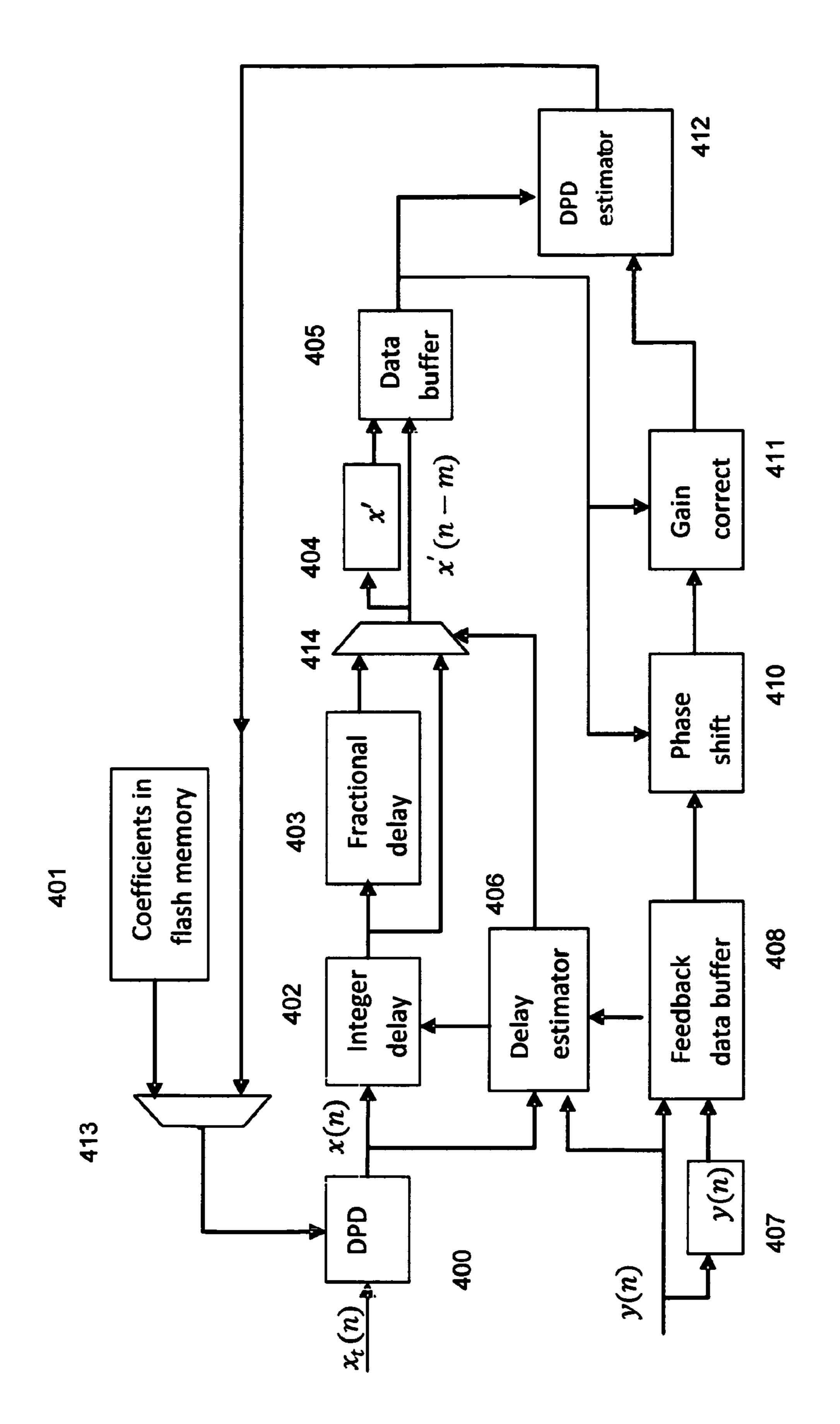
FIG. 4. Digital Predistortion Algorithm
