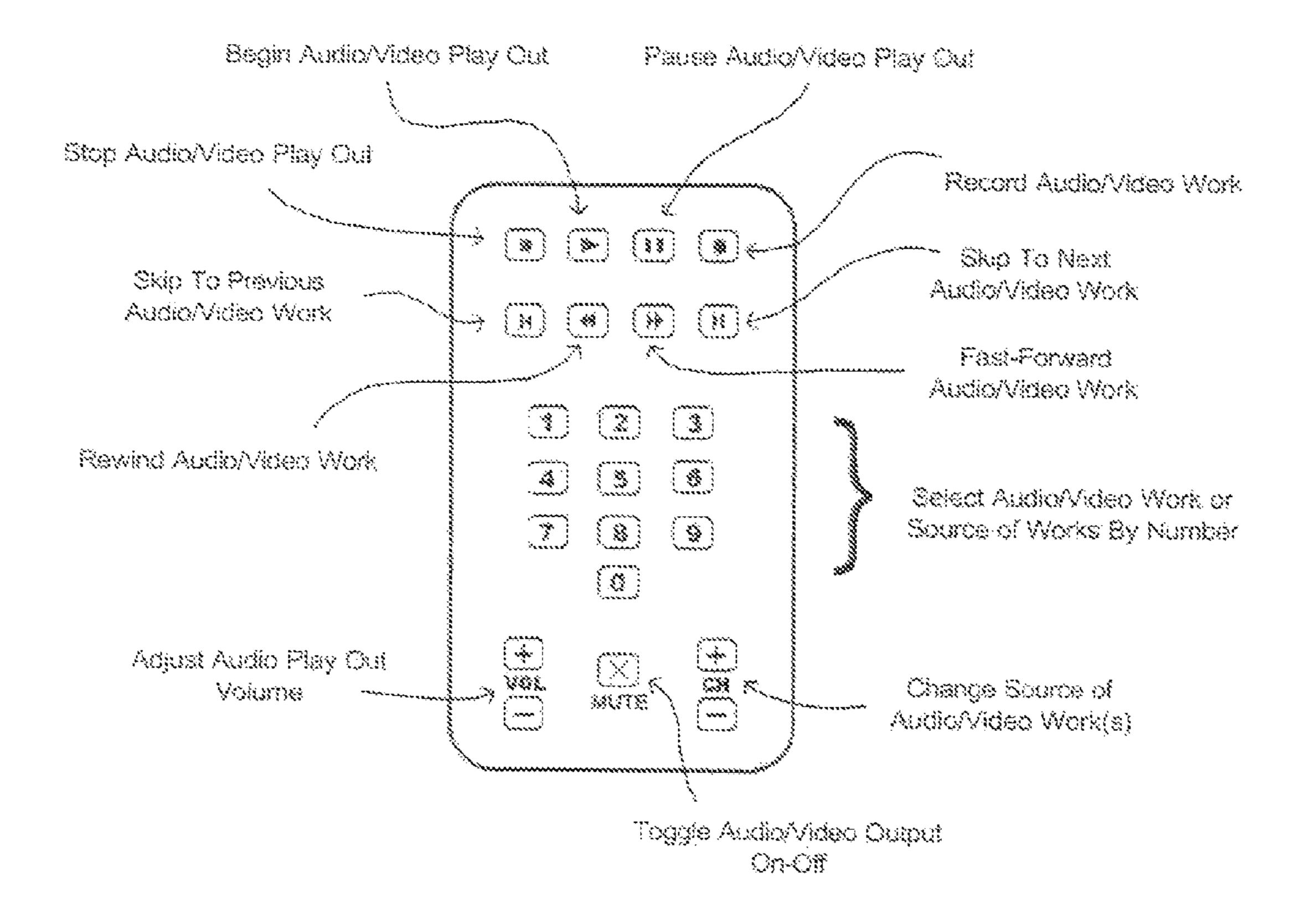
Figure 2. Hand-Held Keypad With Audio/Video Play Out Control Keys
