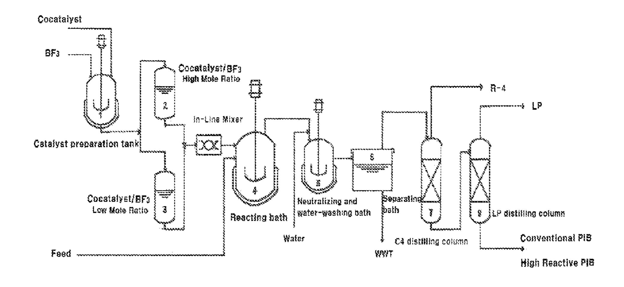
controlling the storage and supply of the low-activity complex catalyst; and a reactor to which reaction raw materials including the high-activity complex catalyst, the low-activity complex catalyst, and isobutene are supplied to be polymerized into highly reactive polybutene.
