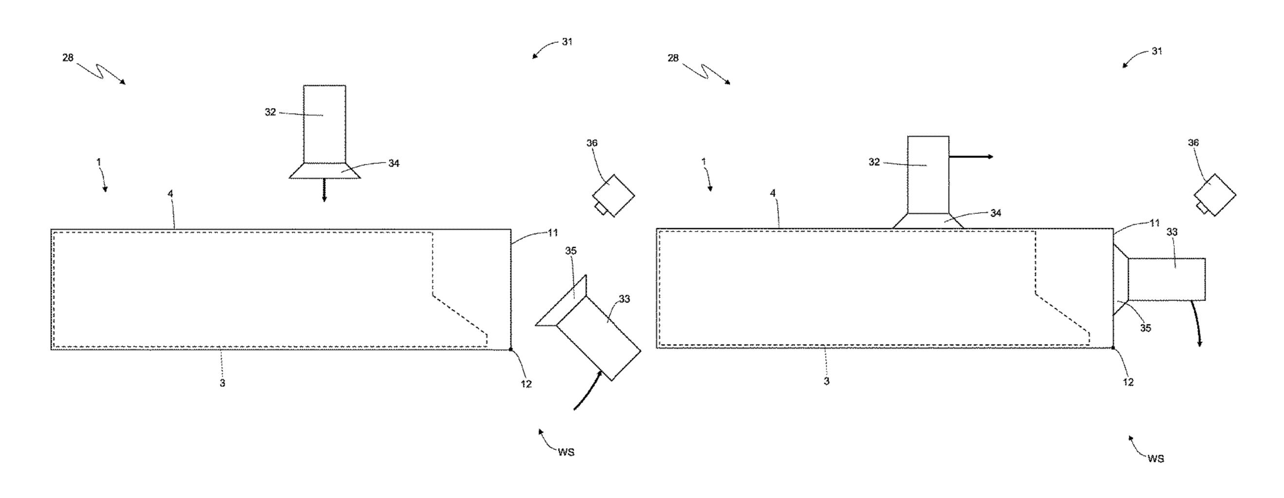
suction head which engages the top wall by suction; and, simultaneously and in coordination with the step of exerting pull on the lid, exerting thrust on an inner container of the package, to slide the inner container axially with respect to the outer container, by means of a second actuator, which contacts a wall of the inner container through a window formed through a corresponding wall of the outer container.
