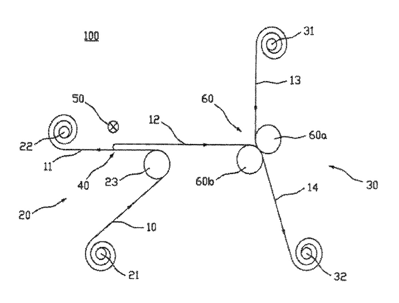
pulled off at the film delaminating station in the direction opposite the running direction of the first laminated strip at said station.
