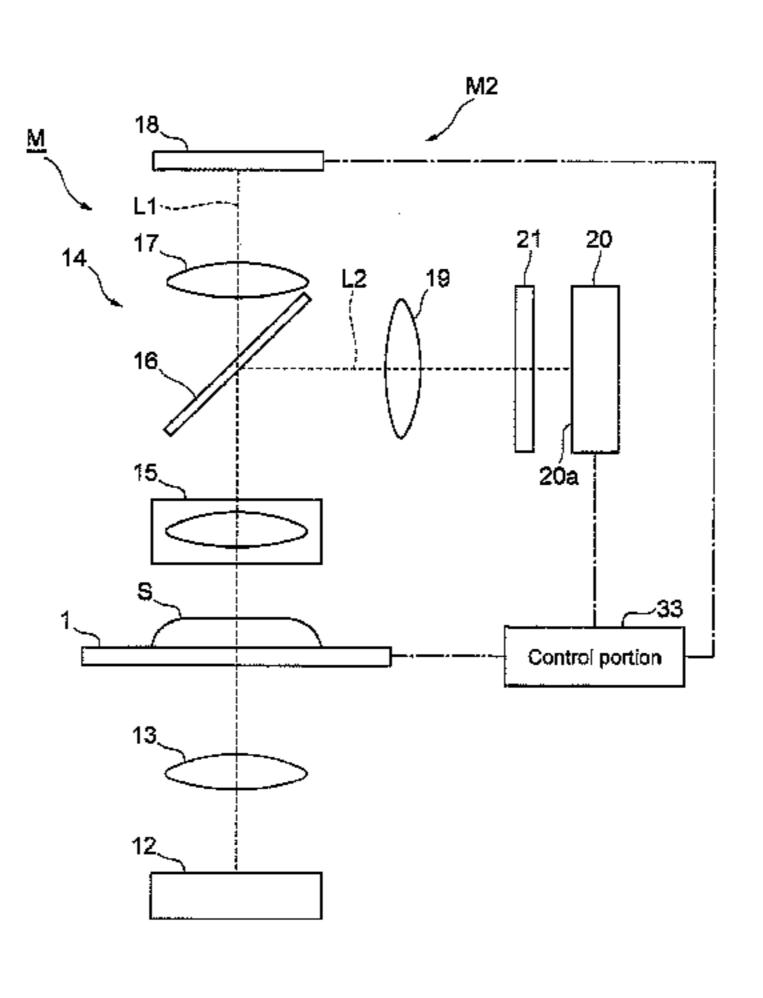
the imaging area of the second imaging device are positioned on the front side of the imaging area in a scanning direction of the sample with respect to the region into which an optical image is made incident which is conjugate to the first optical image made incident into the first imaging device. Thereby, it is possible to obtain in advance a deviation direction of a focus position of the objective lens by a simple constitution.
