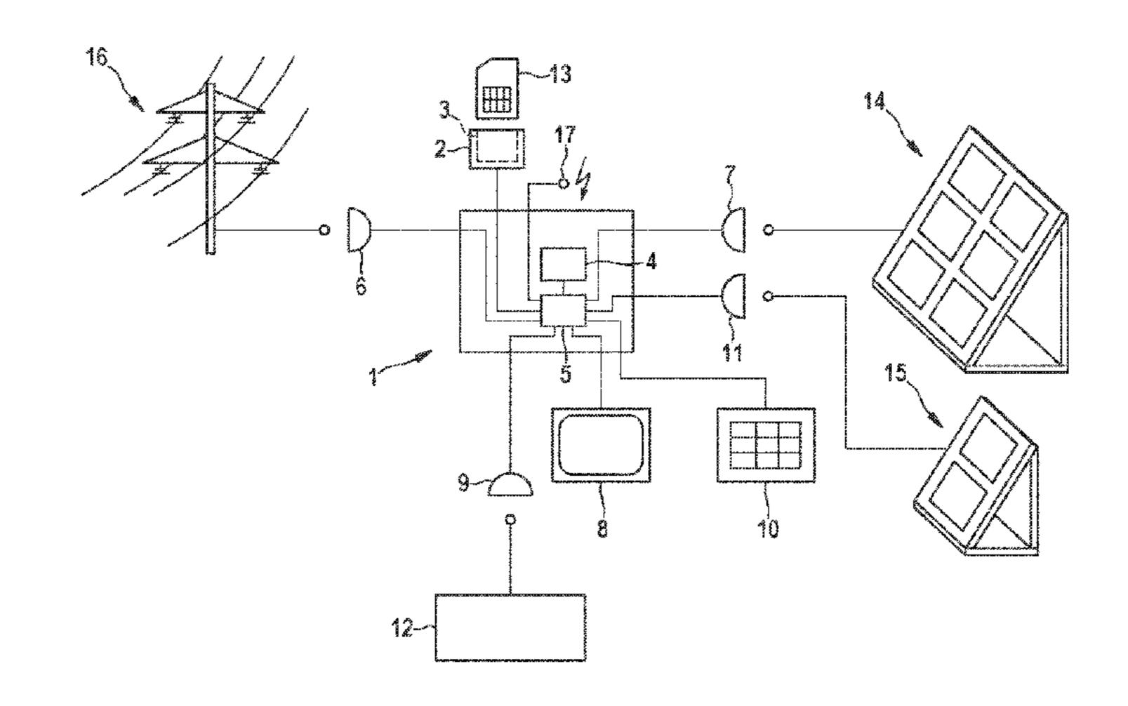
start-up of the power converter in accordance with the settings data, the settings data being read from the exchangeable external memory medium. A method for setting the operation and/or the start-up of a power converter, for example, for setting the operation and/or the start-up of an inverter, is performed in accordance with settings data read from an external memory medium.
