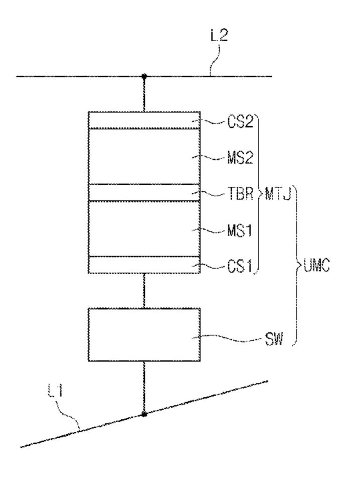
two free layers with different thicknesses can enable a magnetic memory device that has increased MR ratio and reduced switching current.
