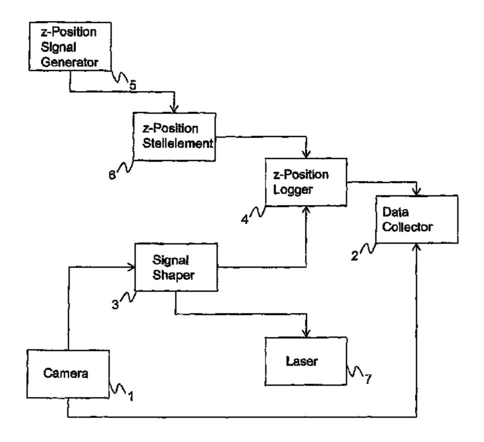
transmits said position to the image capture circuit, which links the position of the specimen in the depth direction to the data of the imaging of a frame such that a threedimensional tomographic image of the specimen can be created.
