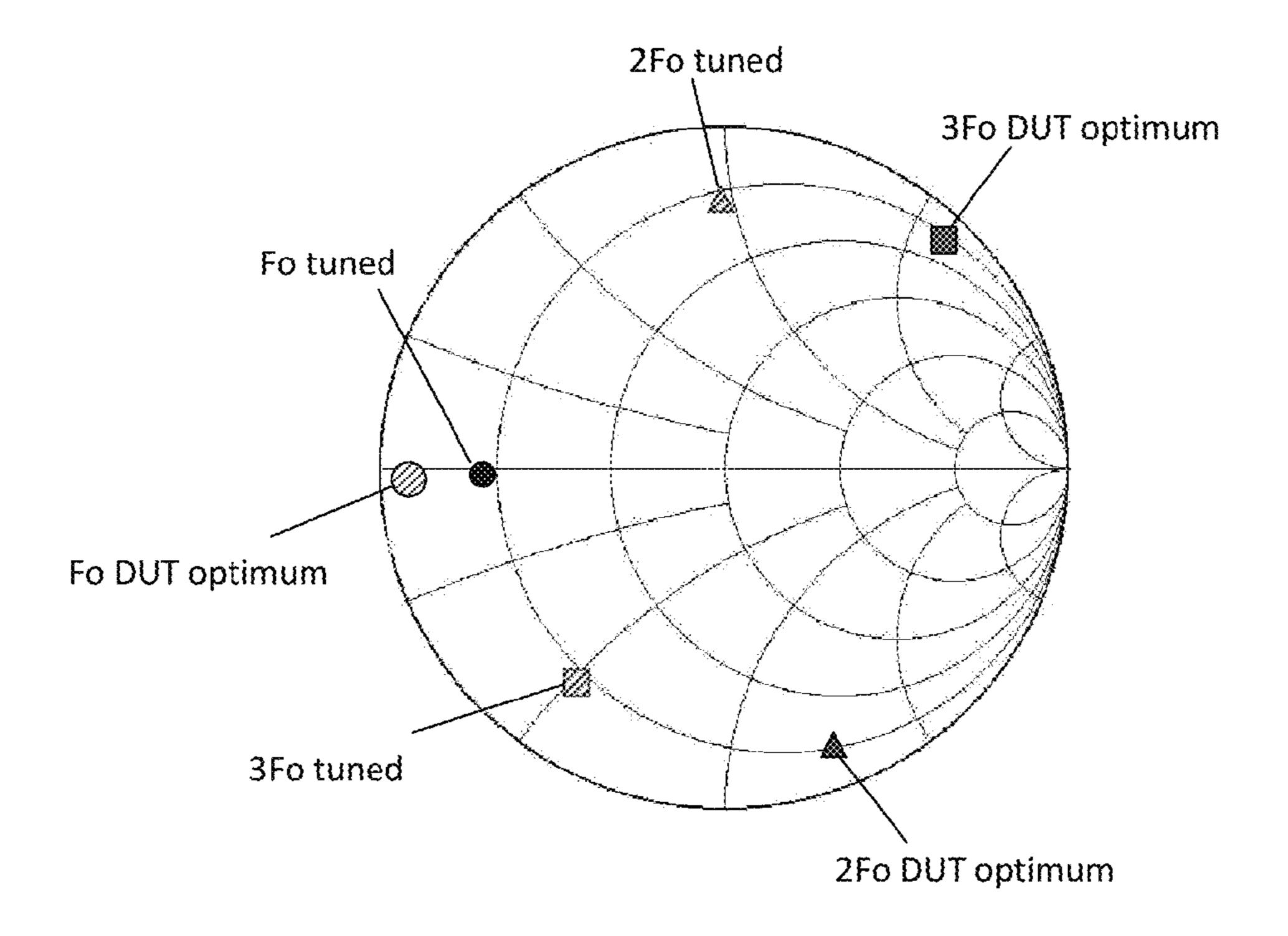
Figure 4: Prior art: harmonic impedances of wideband tuner (tuned for Fo)
