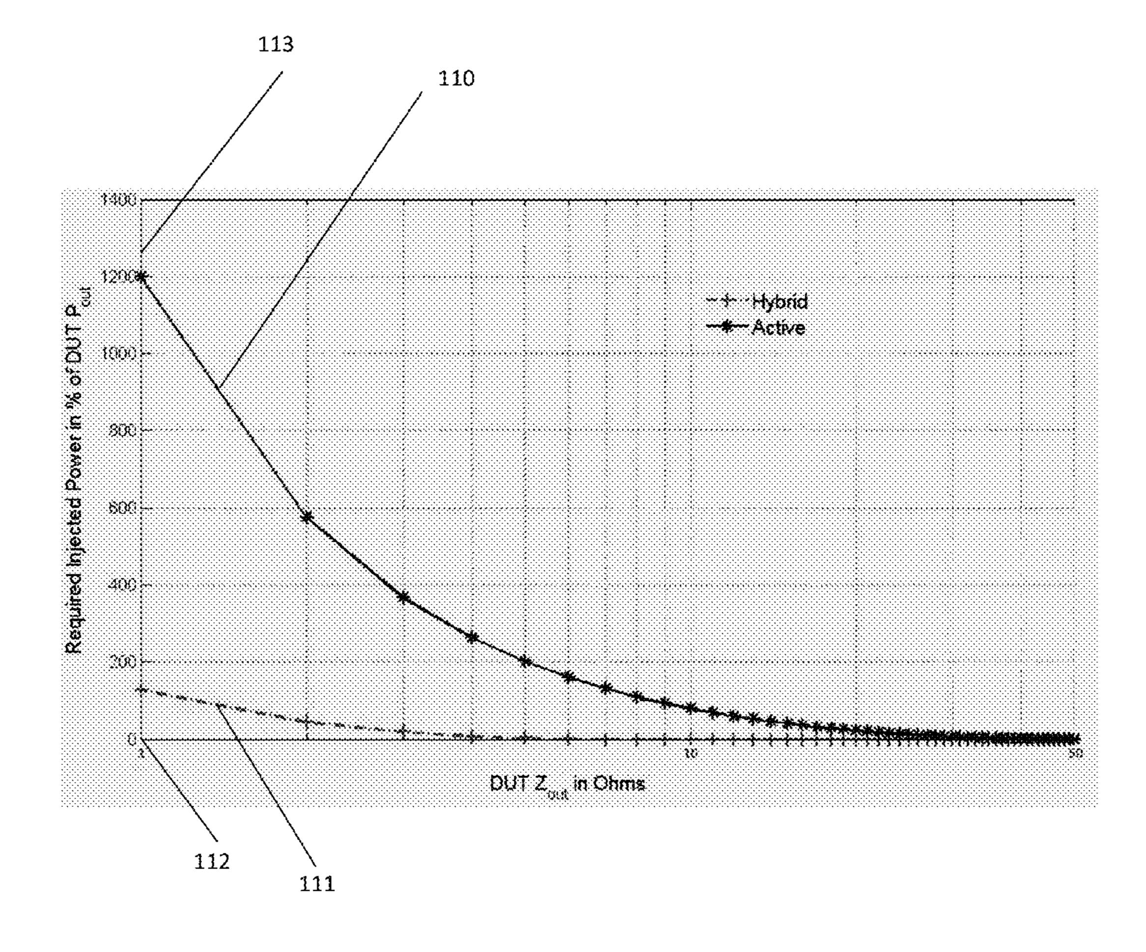
Figure 11: Reduced injection power due to passive pre-matching (hybrid)
