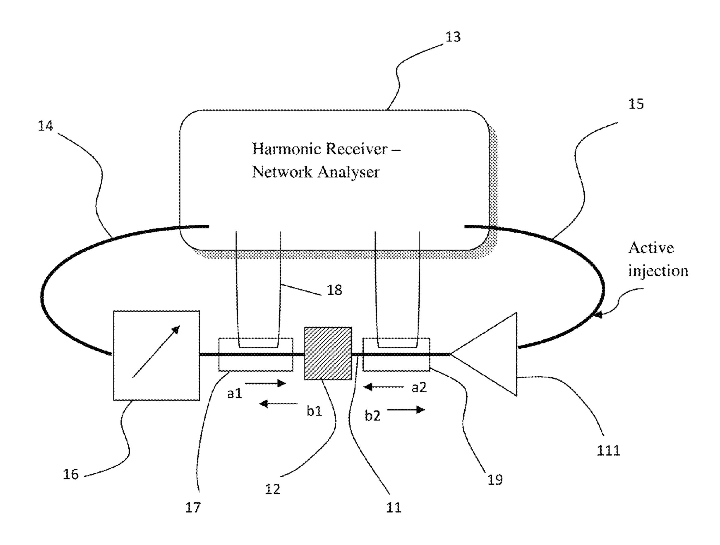
Figure 1: Prior art, active injection load pull
