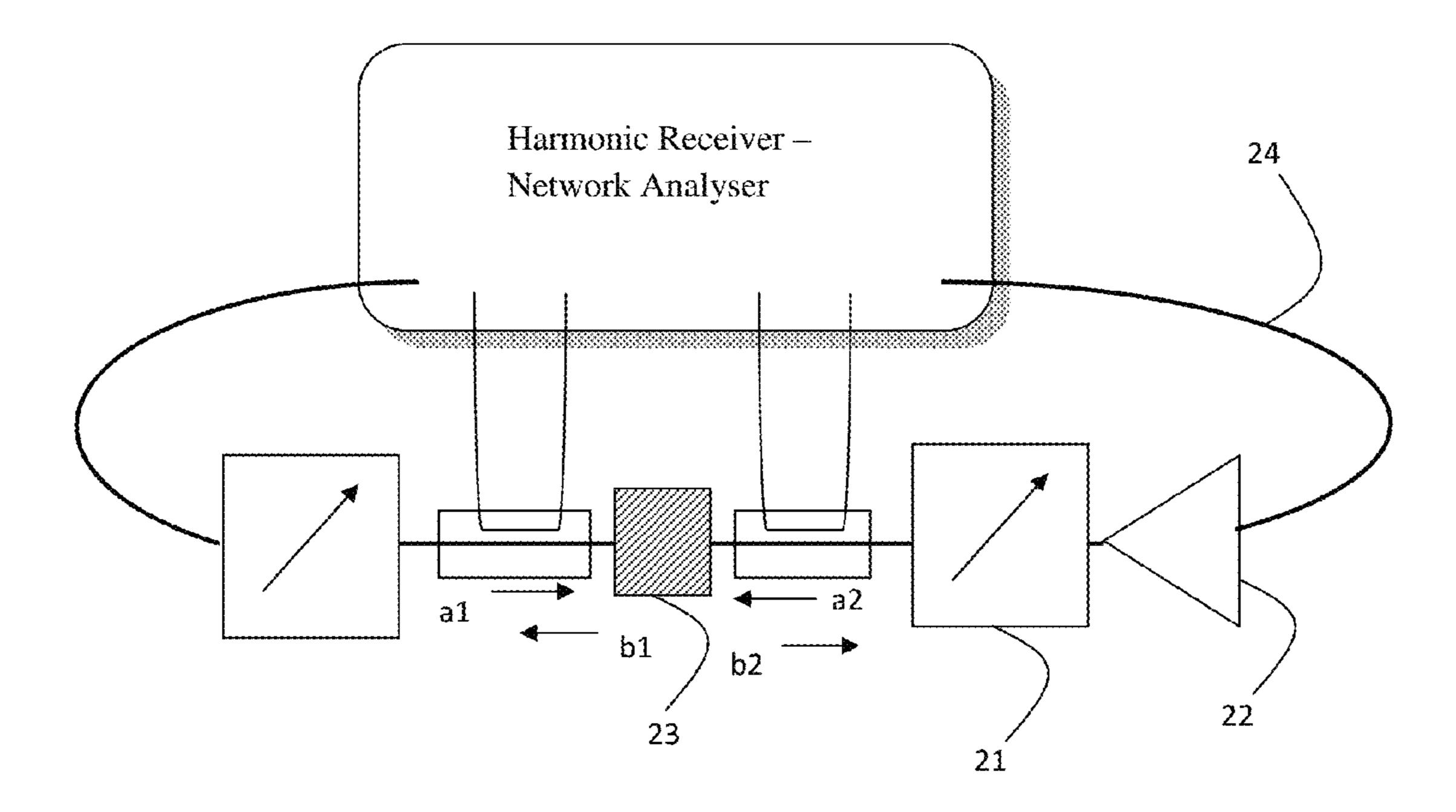
Figure 2: Prior art, active injection load pull using pre-match tuner
