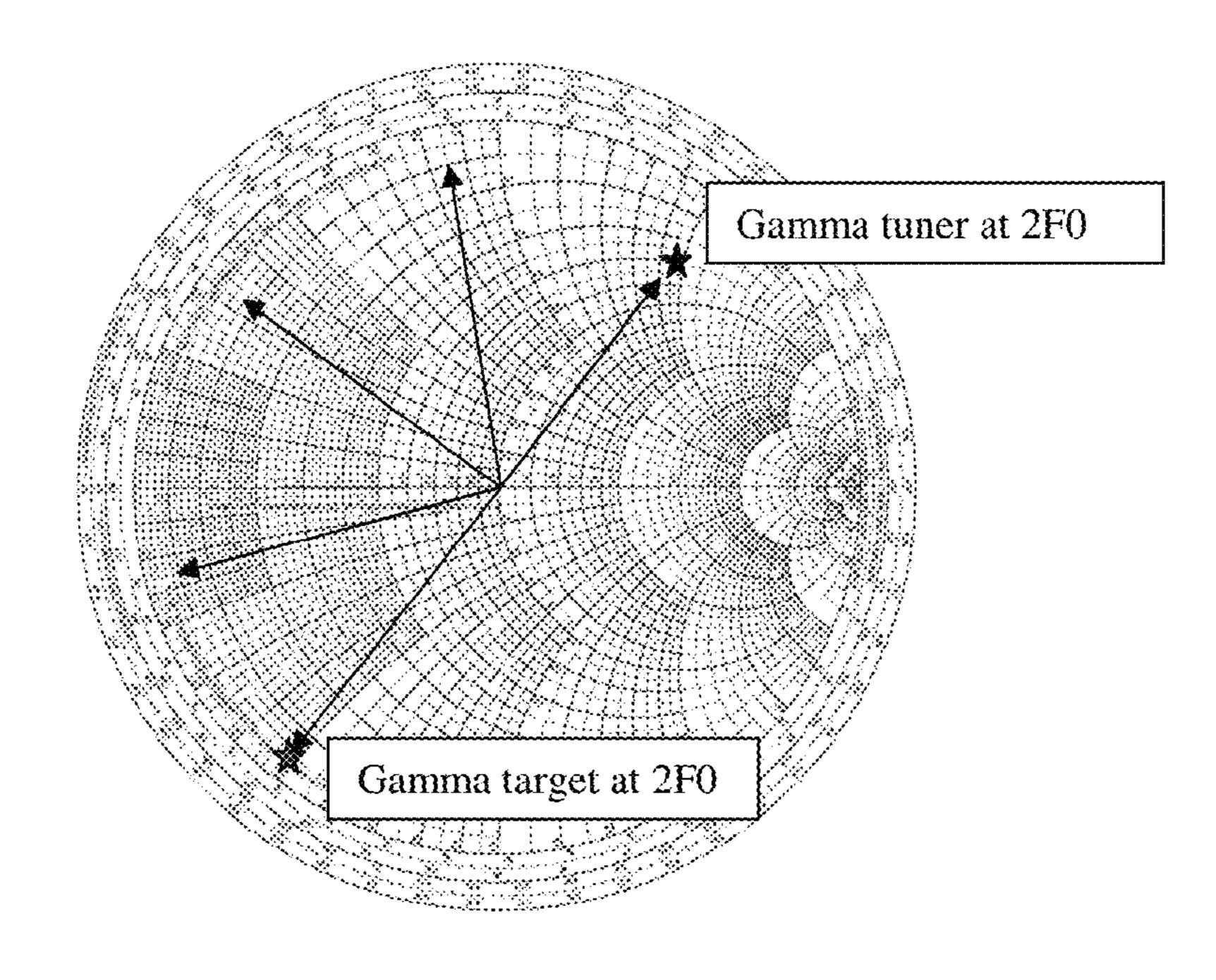
Figure 6: Prior art; mismatch tuning with wideband tuner (possible scenario)
