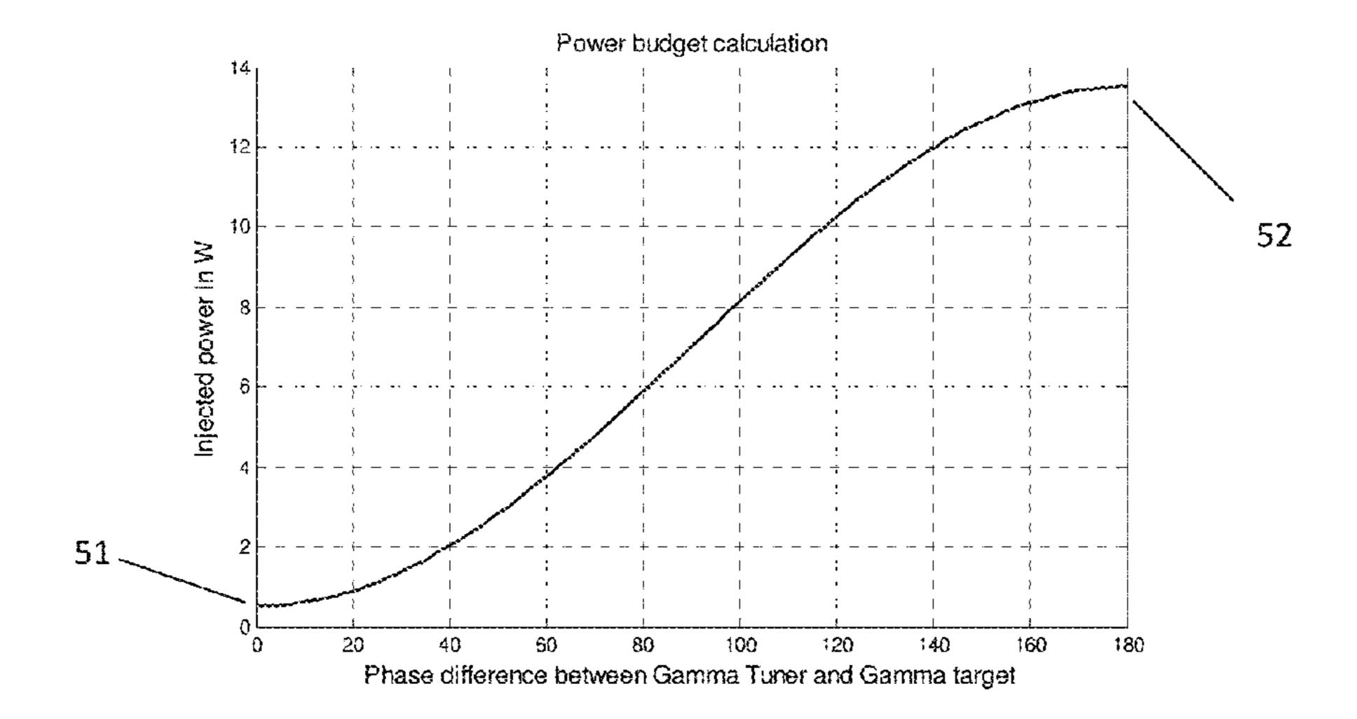
Figure 5: Prior art, power requirement as a function of phase difference between tuned and target points
