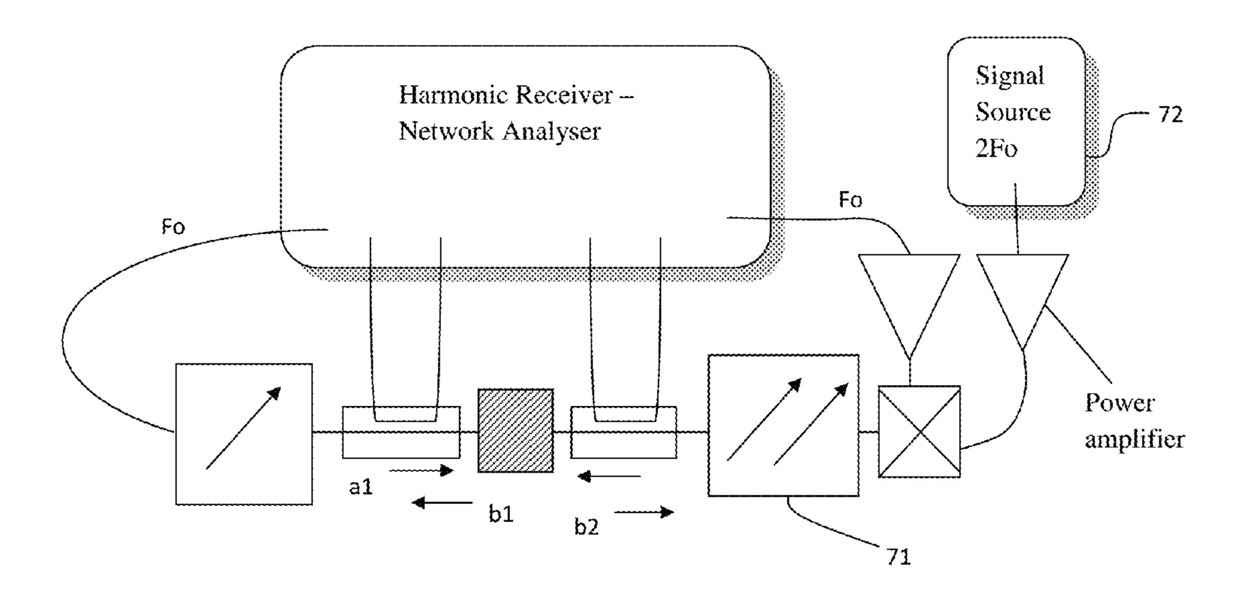
Figure 7: Active injection load pull using two sources and harmonic tuner
