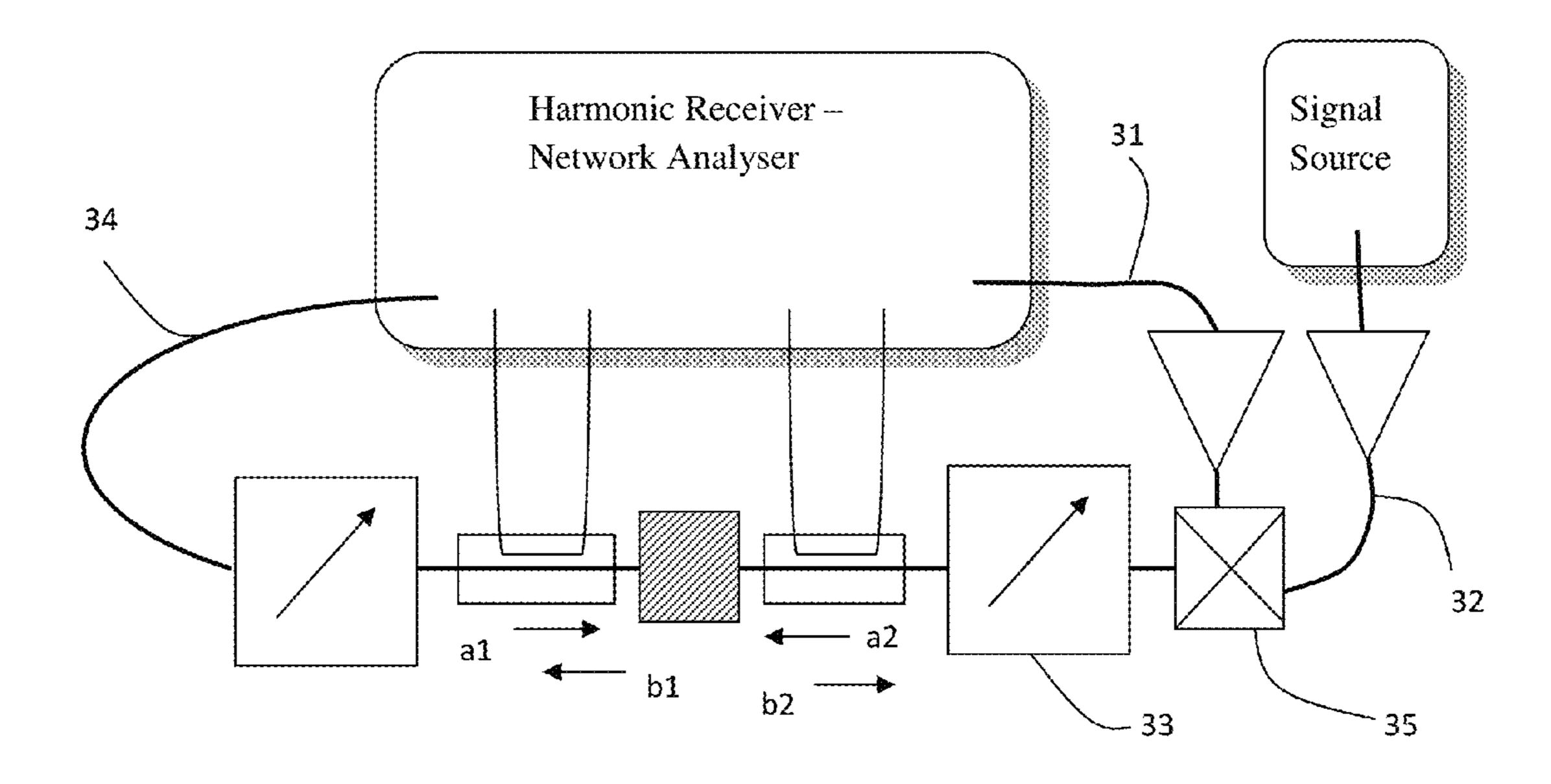
Figure 3: Prior art, active injection load pull using two sources and pre-match tuner
