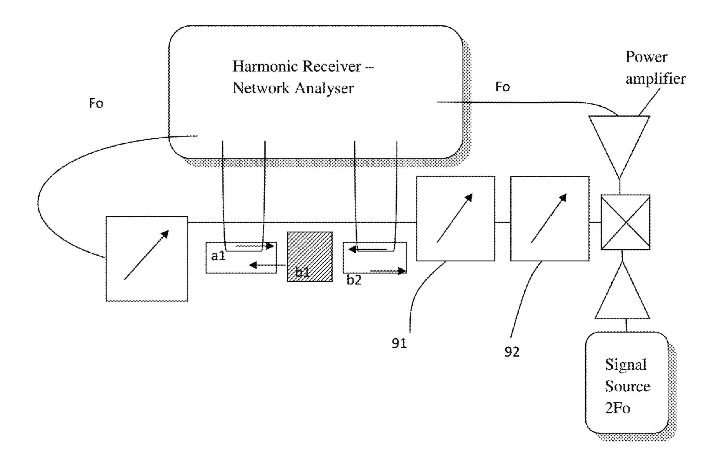
Figure 9: Active injection load pull using two sources and cascade of tuners
