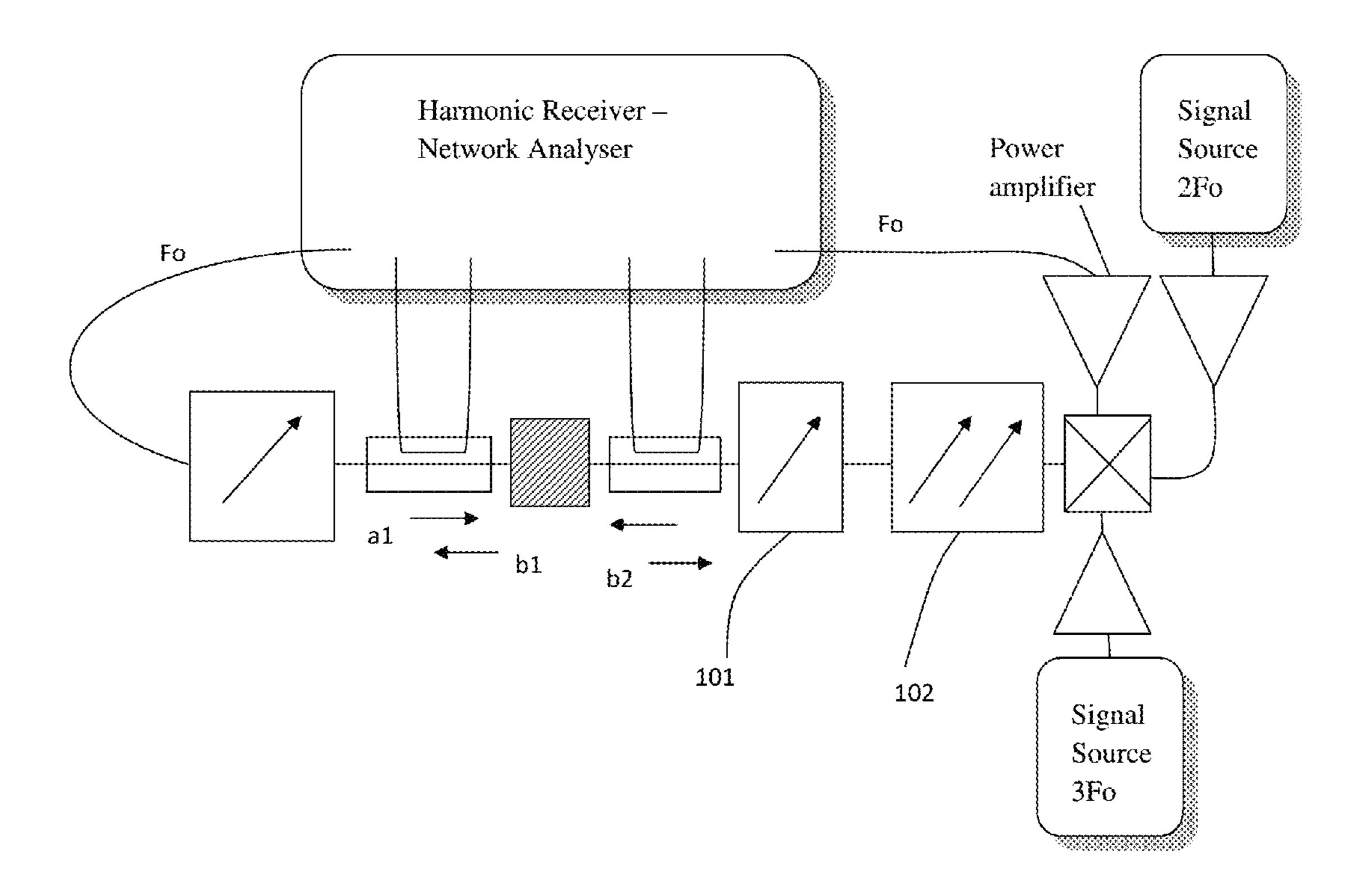
Figure 10: Active injection load pull using three sources and cascade of tuners
