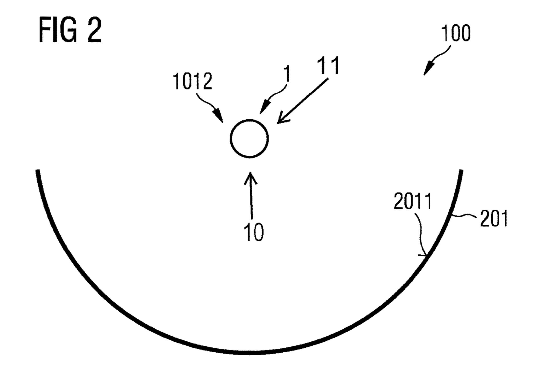
HEAT RECEIVER TUBE, METHOD FOR MANUFACTURING THE HEAT RECEIVER TUBE, PARABOLIC TROUGH COLLECTOR WITH THE RECEIVER TUBE AND USE OF THE PARABOLIC TROUGH COLLECTOR
