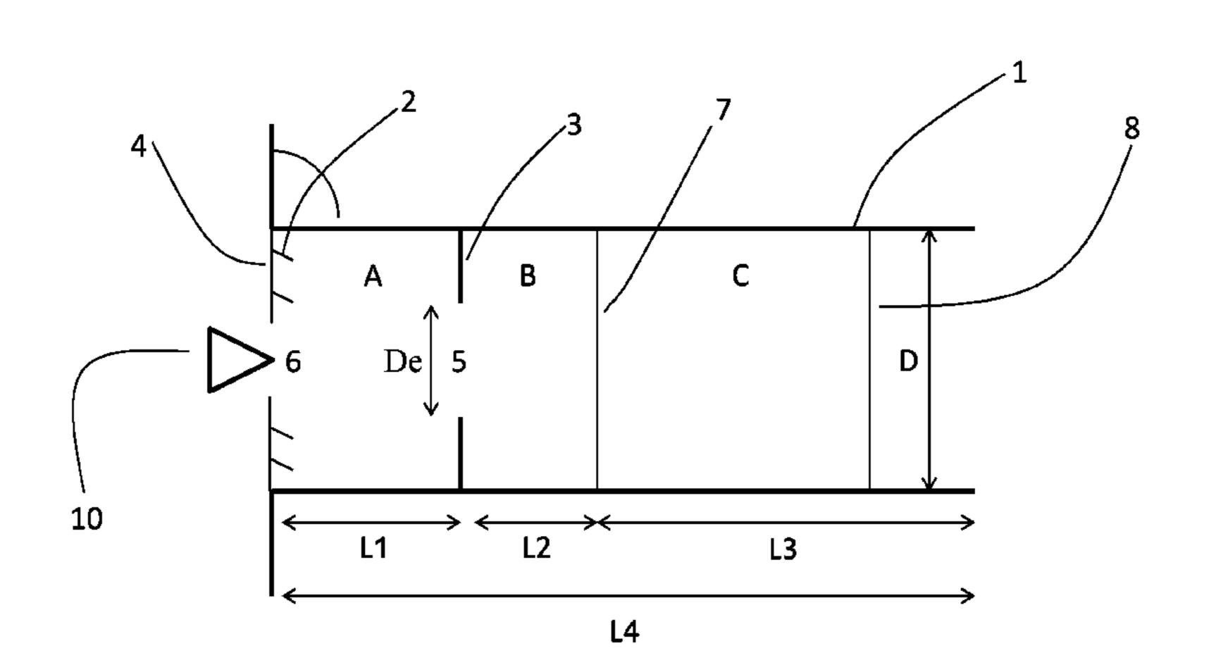
combustion body is <0.7 and the constrictor plate is placed at a distance (L1) from the base of the swirler base so that L1/De>1. A primary mixing plate is placed downstream from the constriction plate at a distance (L2) so that the ratio L2/L1<1 to allow maximum mixing of the homogeneous combustion.
