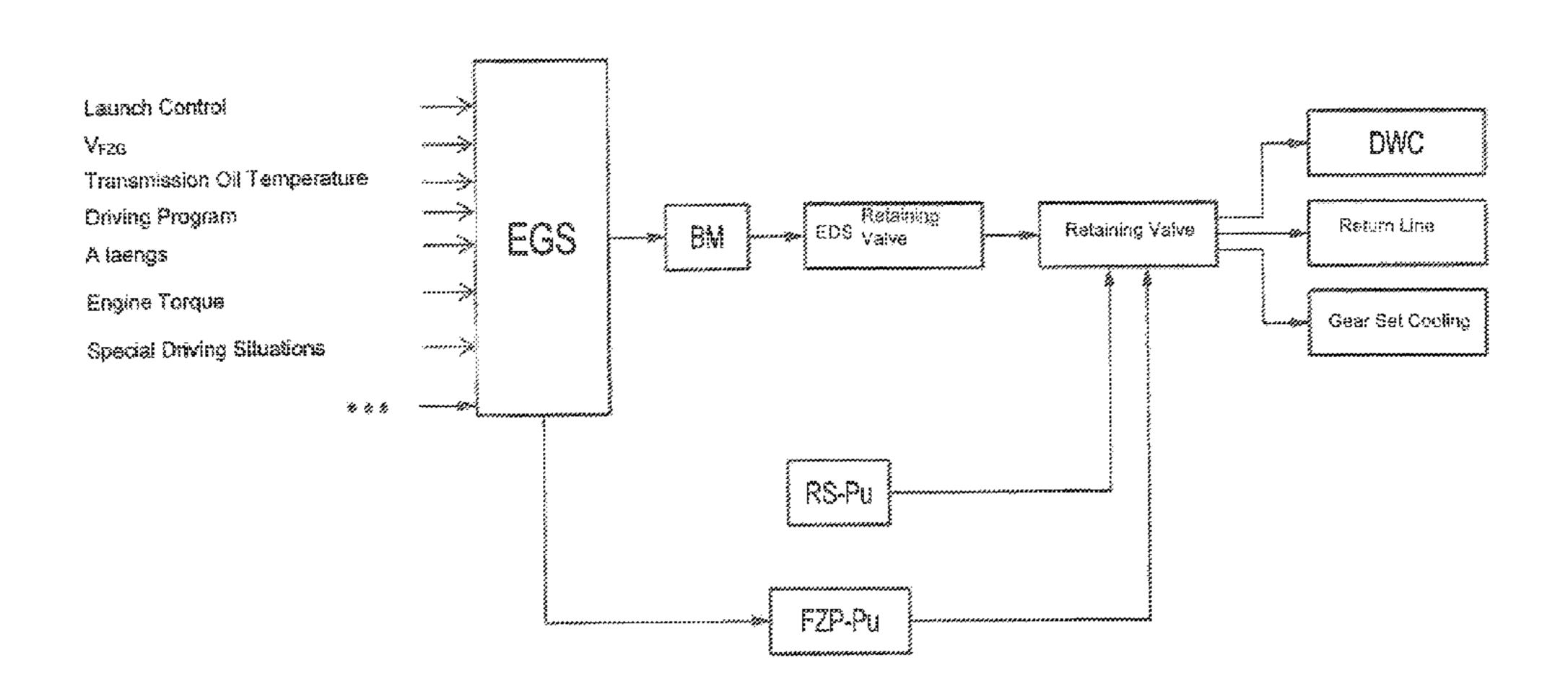
distribution with the hydraulic pump controlled on the engine side and the hydraulic pump controlled on the gear set side.
