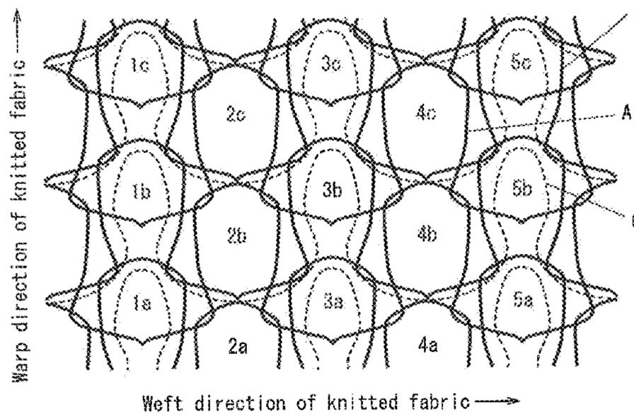
the stretching force in the warp direction to that in the weft direction is 0.5 to 1.8; and the elongation recovery percentages of elongation in the warp and weft directions are 85% or more as determined after subjecting the fabric to three 80% elongation/recovery cycles.
