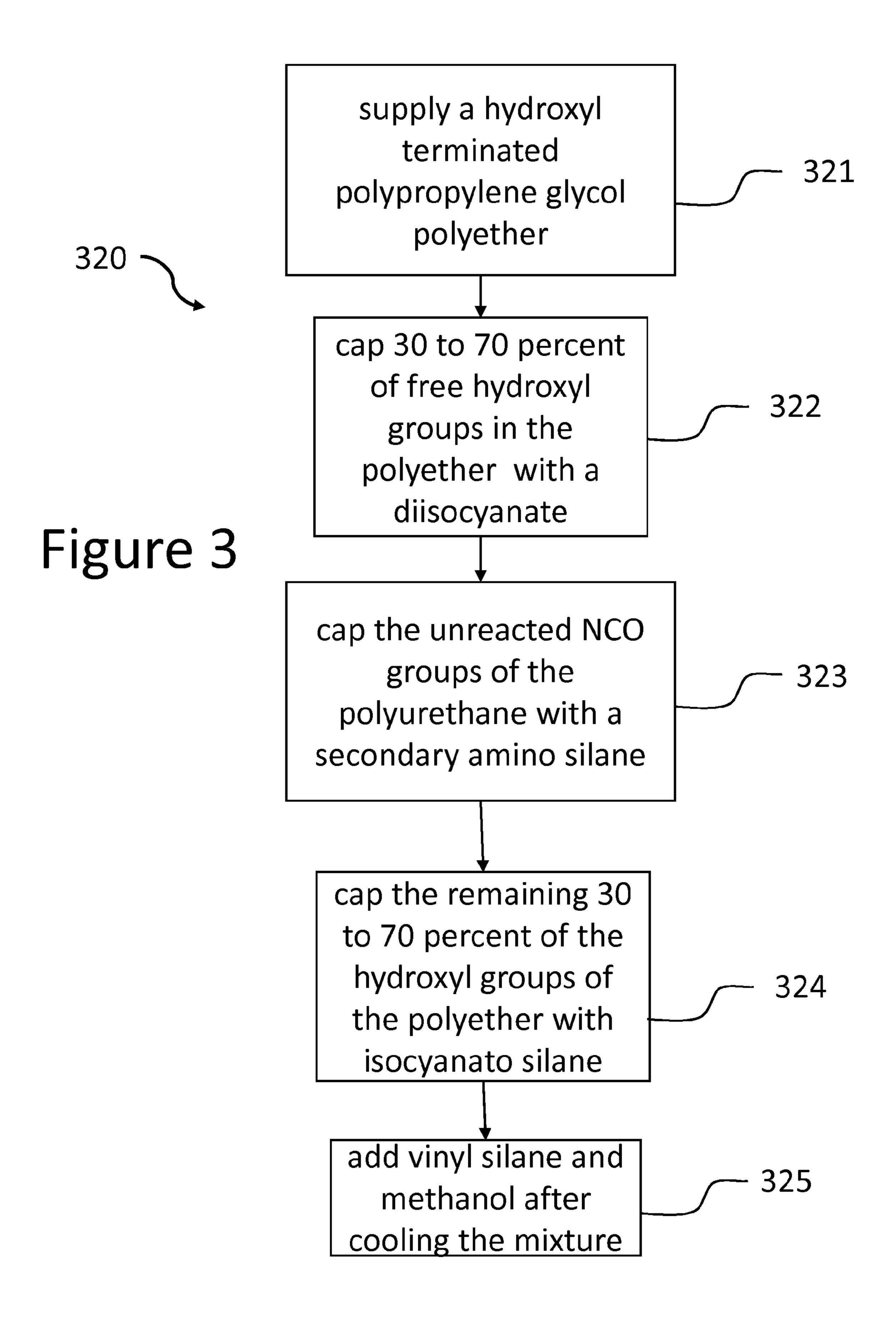
LOW VISCOSITY DIMETHOXY AMINO SILANE POLYURETHANE WITH TRIETHOXY SILYL GROUPS FOR SEALANTS AND ADHESIVES WITH EASY PROCESSING, HIGH TENSILE STRENGTH AND LOW METHANOL EMISSIONS ON CURING
