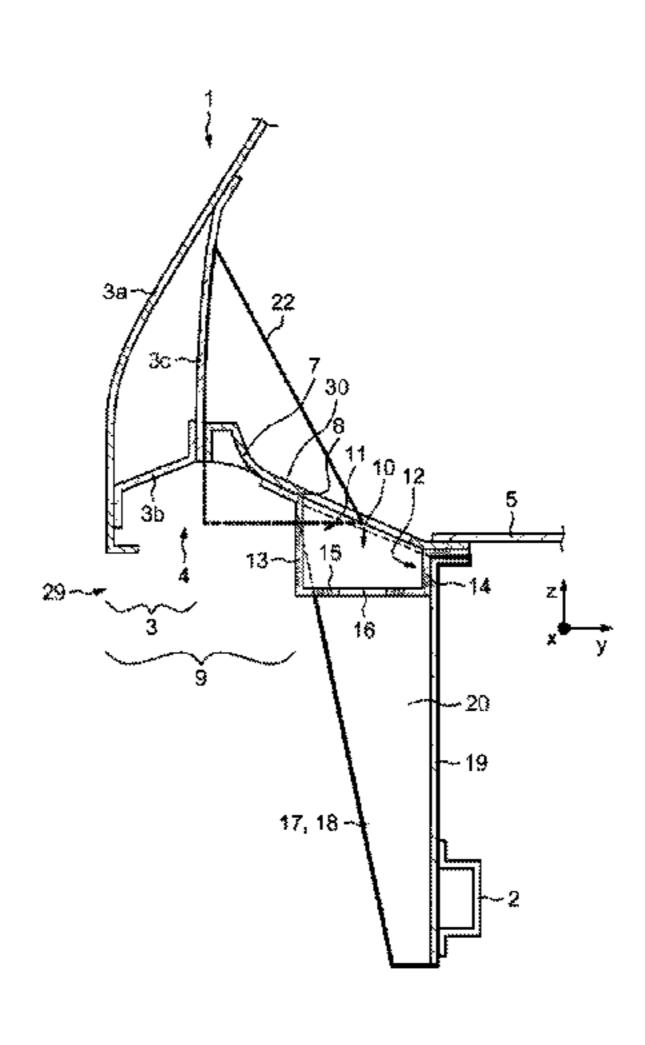
oblique surface portion around and beyond the edges of the mount. The superstructure also includes a structural plate rigidly connected to an oblique surface portion of the wheel arch housing part and secured to a substantially vertical surface portion of the superstructure.
