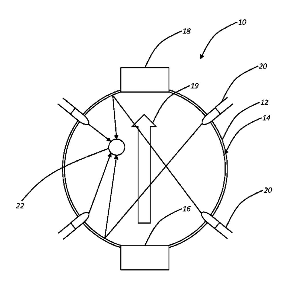
exemplary embodiment, the flow cell is an integrating sphere. Optionally, the system also includes a photocatalyzing material disposed on at least a portion of the interior surface of the flow cell.
