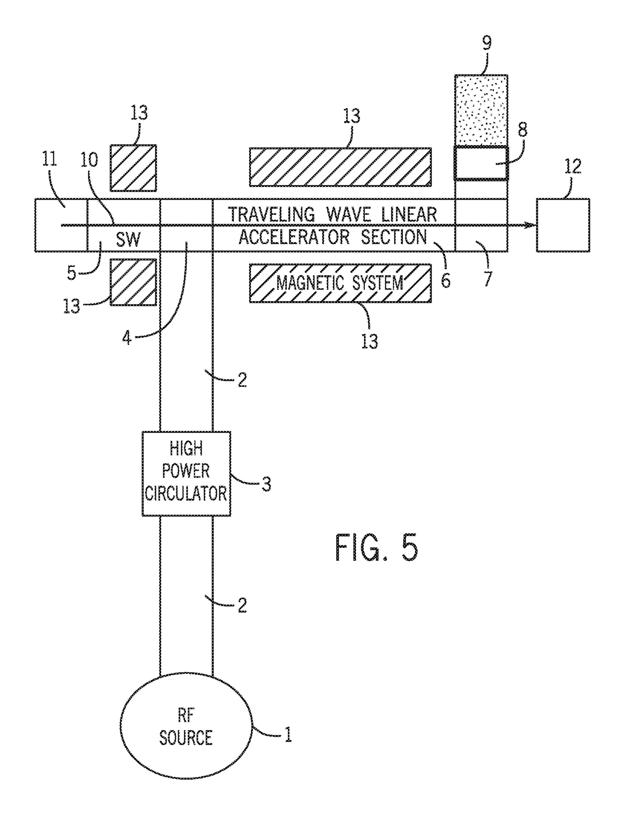
HYBRID LINEAR ACCELERATOR WITH A **BROAD RANGE OF REGULATED** ELECTRON AND X-RAY BEAM PARAMETERS INCLUDES BOTH STANDING WAVE AND TRAVELING WAVE LINEAR SECTIONS FOR PROVIDING A MULTIPLE-ENERGY HIGH-EFFICIENCY ELECTRON BEAM OR X-RAY BEAM USEFUL FOR SECURITY INSPECTION, NON-DESTRUCTIVE TESTING, RADIATION THERAPY, AND OTHER APPLICATIONS
