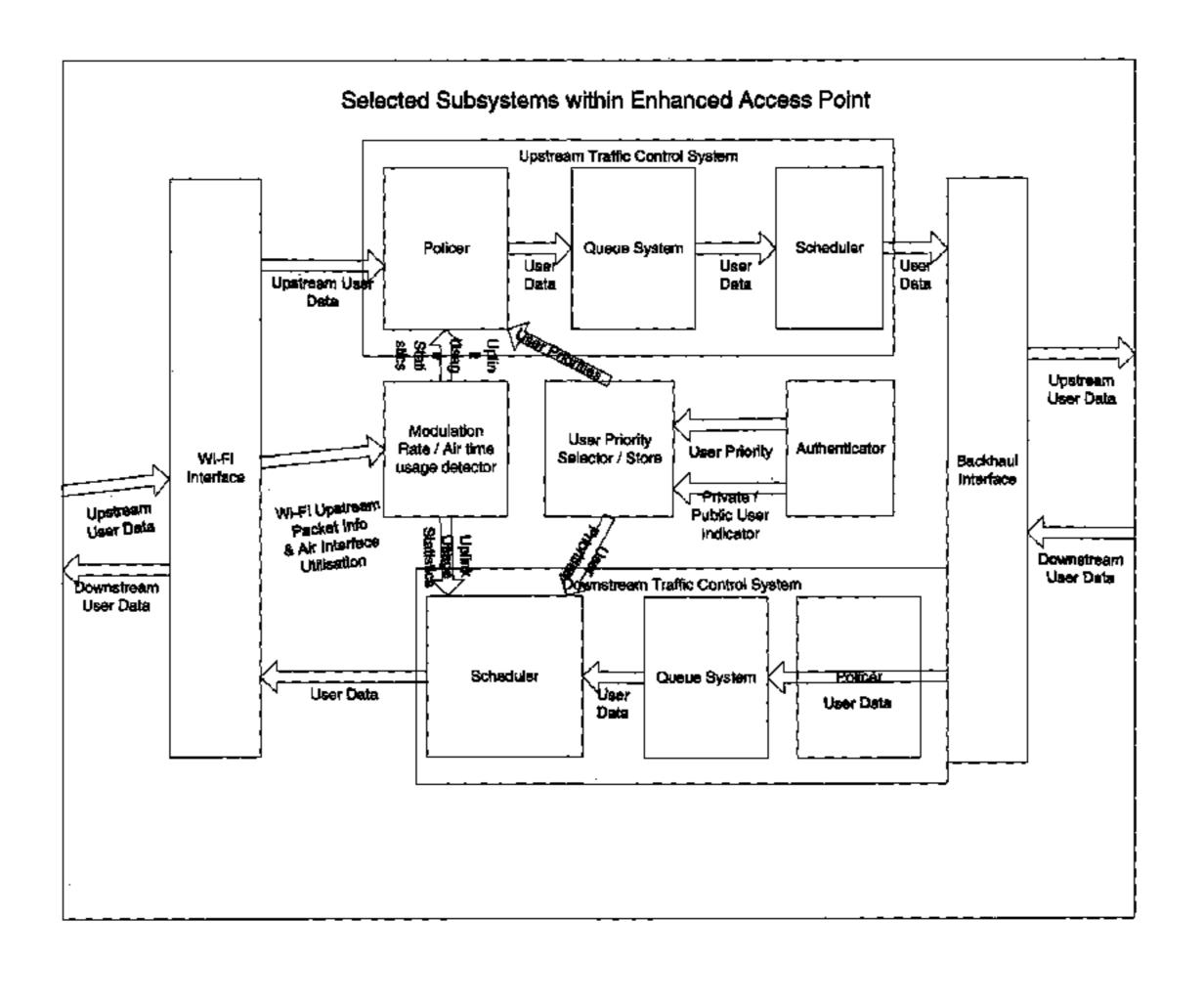
streams to back off when they detect packet loss). Finally, for some embodiments where public Wi-Fi is being delivered through private Wi-Fi access points, the traffic control system is to manage the air interface utilization split between public and private WiFi users, to ensure that private users do not have their Wi-Fi air interface network capacity unduly impaired by public users.
