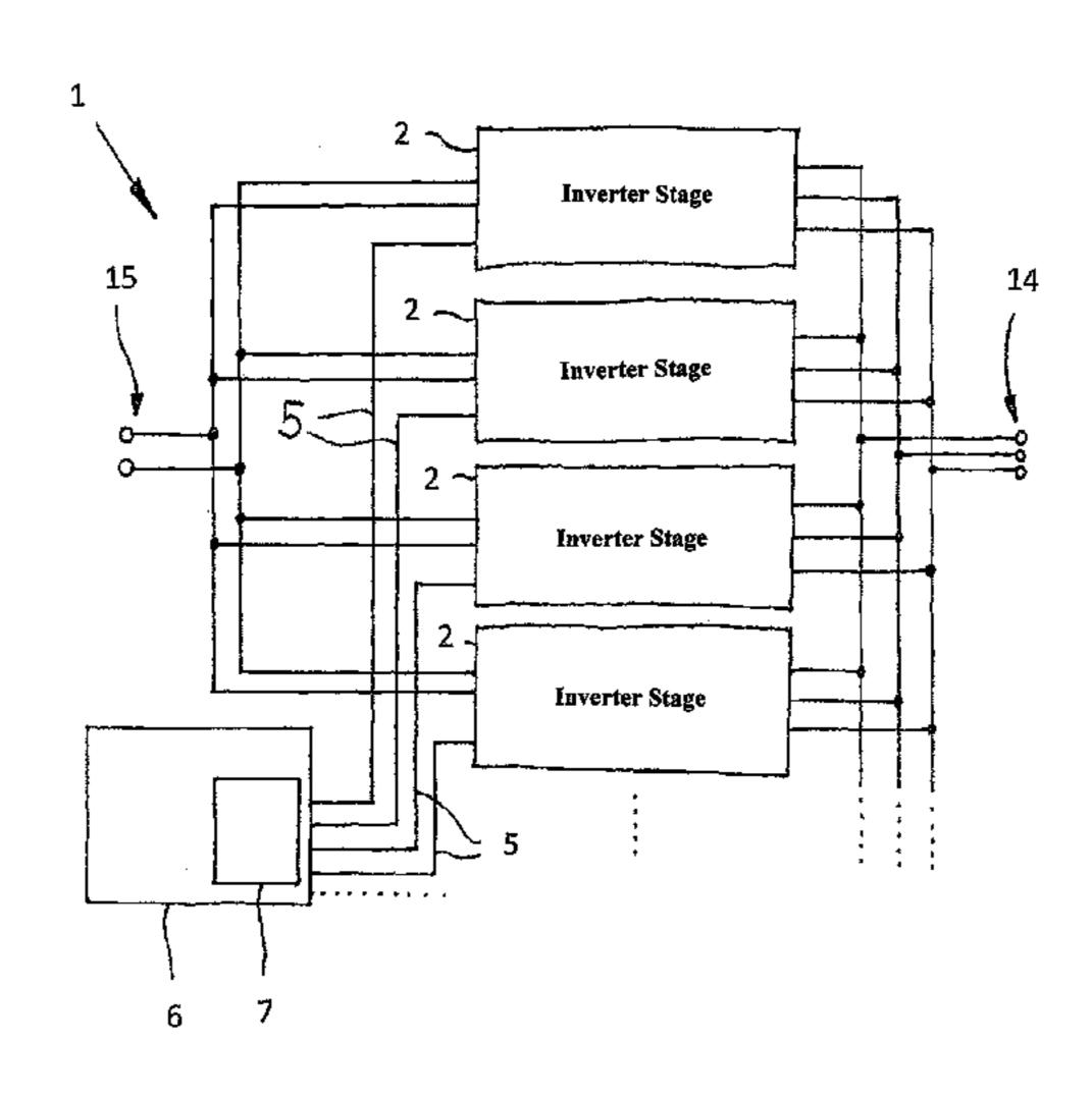
actuation of the switching elements (3) of the inverter stages (2) in a sufficiently rapid way on the other hand in order to avoid impairing the quality of the output current formed by the inverter stage (2).
